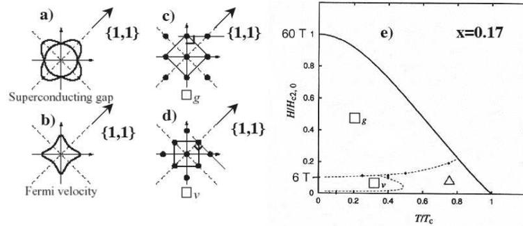
**Figure 3.** Both d-wave superconducting gap (panel a) and Fermi velocities (panel b) anisotropies will result in square lattices (panels c–d), but with different orientations with respect to the gap nodes. The resulting phase diagram taken from Nakai *et al* [8] for optimally-doped LSCO is given in panel e.
