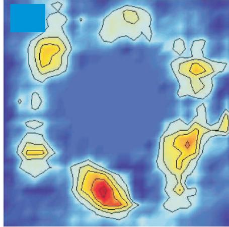
**Figure 4.** Small angle neutron diffraction pattern showing the existence of an ordered vortex phase at low fields (150 Oe) and temperature (6.2 K). The intensity of this pattern rapidly falls as the field is increased towards the vortex-glass phase [14].
