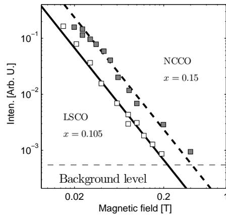
**Figure 6.** Integrated intensity as a function of applied magnetic field for LSCO  $x = 0.10$  and NCCO (dashed line). Notice that both axis are logarithmic. The solid and dashed line are  $I \sim H^2$  [14].
