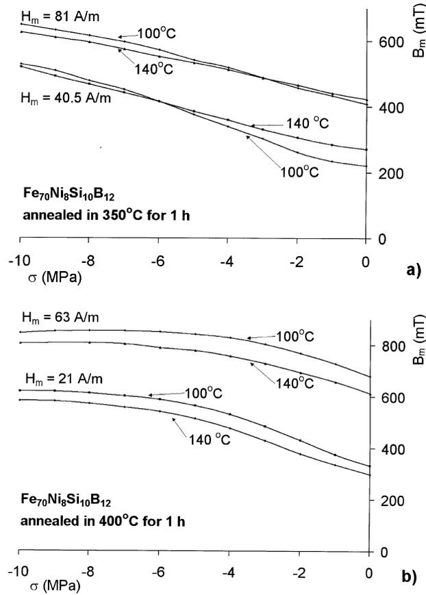
**Figure 4.** The temperature dependence of magnetoelastic characteristics  $B(\sigma)_{H_m}$  of Fe<sub>70</sub>Ni<sub>8</sub>Si<sub>10</sub>B<sub>12</sub> amorphous alloy cores annealed at (a) 350°C and (b) 400°C for 1 h.
