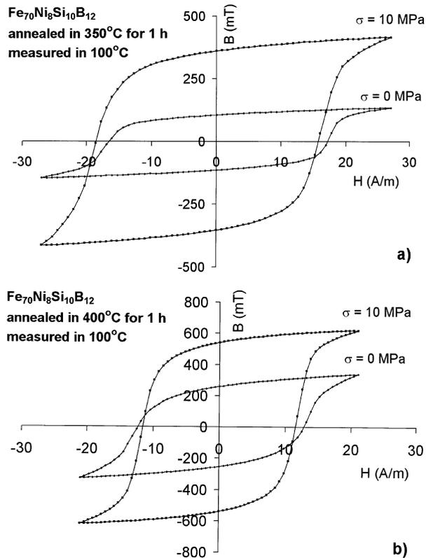
**Figure 3.** The influence of compressive stress  $\sigma$  on the magnetic hysteresis loop  $B(H)_\sigma$  of  $Fe_{70}Ni_8Si_{10}B_{12}$  amorphous alloy cores annealed at (a) 350°C and (b) 400°C for 1 h (measured at 100°C).
