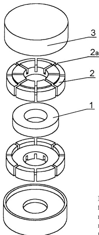
**Figure 1.** Schematic diagram of the device for applying uniform compressive stress to the ring core [12]. (1) Investigated ring core, (2) non-magnetic cylindrical backing, (2a) grooves for windings, (3) base backings.
