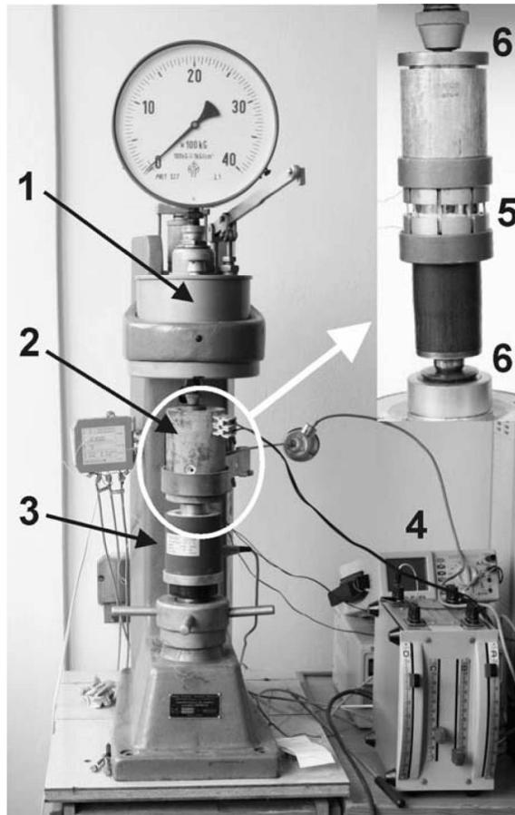
**Figure 2.** System for magnetoelastic tests of ring-shaped cores: (1) hydraulic press, (2) resistive furnace with device presented in figure 1, (3) strain-gauge force transducer, (4) furnace control unit, (5) core in backings (as presented in figure 1) and (6) ball joints.
