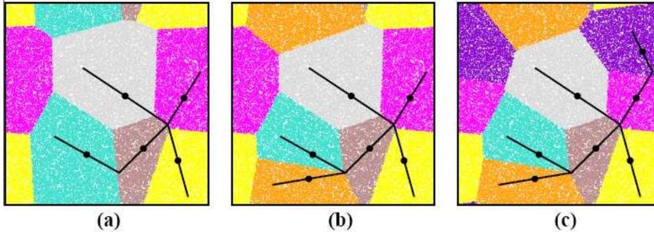
**Figure 3.** The associated Voronoi cells for the growing network: (a) Five links, (b) six links and (c) seven links. The whole space is partitioned into different cells around each link centre.
