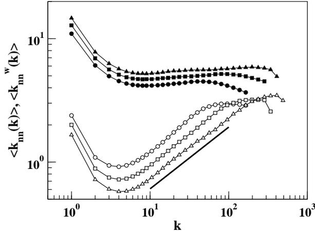
**Figure 5.** The average degree  $\langle k_{nn}(k) \rangle$  and the average weighted degree  $\langle k_{nn}^w(k) \rangle$  of a neighbour of a node of degree  $k$  are plotted with  $k$  with solid and empty symbols for networks with  $m = 1$ . Plots for three different system sizes  $N = 2^{12}, 2^{14}$  and  $2^{16}$  are denoted by circles, squares and triangles respectively. The solid line is guide to the eye having a slope  $1/2$ .
