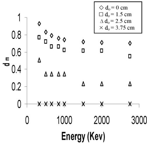
**Figure 5.** Dependence of ratio of source–detector distance to detector radius at which minimum intrinsic efficiency occur on  $\gamma$ -photon energy.
