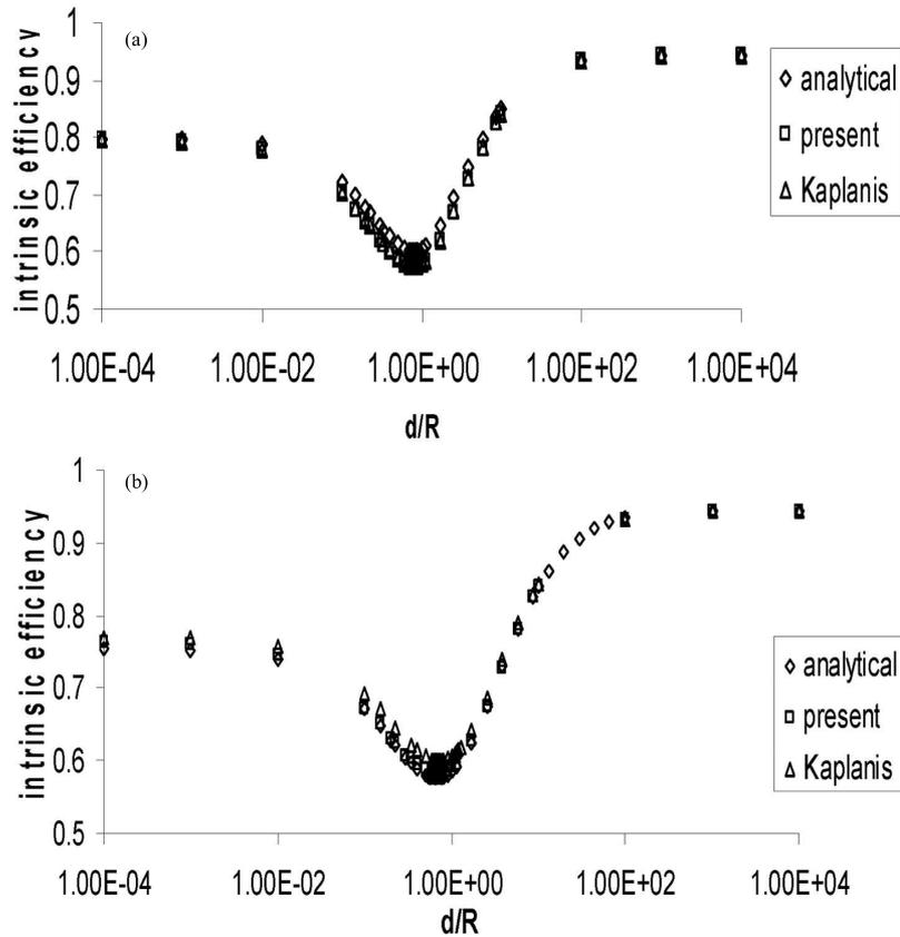
**Figure 3.** Comparison of the analytical method and the Monte Carlo method with the approach of Kaplanis [5] for  $\gamma$ -photon energy 662 keV for two off-axis distances of (a) 0 cm and (b) 1.5 cm.
