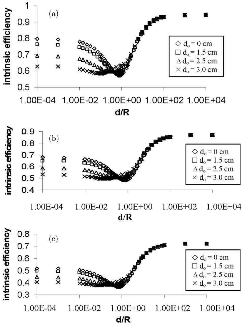
**Figure 4.** Variation of intrinsic efficiency with the ratio of source-detector distance to detector radius at four different off-axis distances for  $\gamma$ -photon with energies (a) 662 keV, (b) 1500 keV and (c) 2750 keV.
