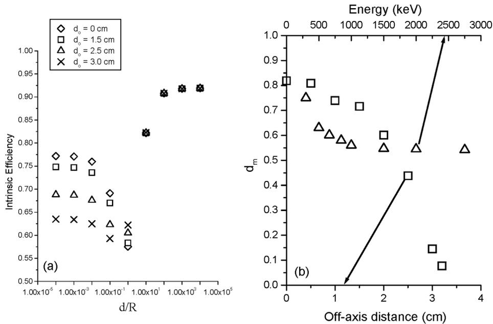
**Figure 7.** Variation of (a) intrinsic efficiency with ratio of source–detector distance to detector radius and (b) ratio of source–detector distance to detector radius at which minimum intrinsic efficiency occur with off-axis distance and energy for a disk source of radius 0.38 cm and thickness 0.1 cm.
