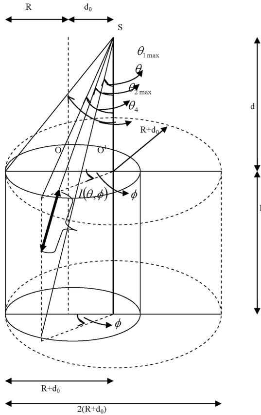
**Figure 2.** Geometrical configuration for the hypothetical detector for punctual  $\gamma$ -photon sampling.
