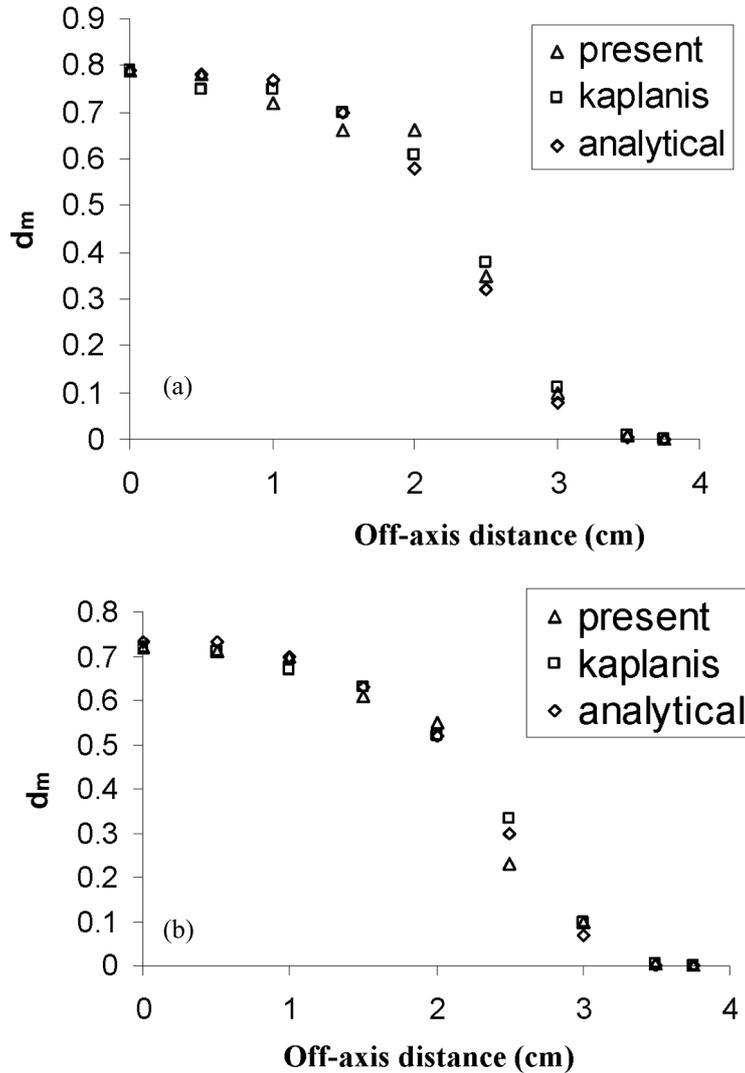
**Figure 6.** Variation of ratio of source–detector distance to detector radius at which minimum intrinsic efficiency occur with off-axis distance for different  $\gamma$ -photon energies (a) 662 keV and (b) 1500 keV.
