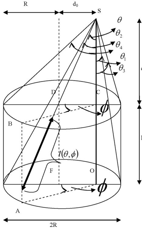
**Figure 1.** Geometrical configuration of the punctual source at off-axial distance above the bare-surface NaI(Tl) detector.
