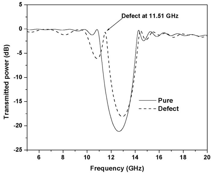
Figure 2. Theoretical simulation of the transmission spectra for the pure and defect structures.
