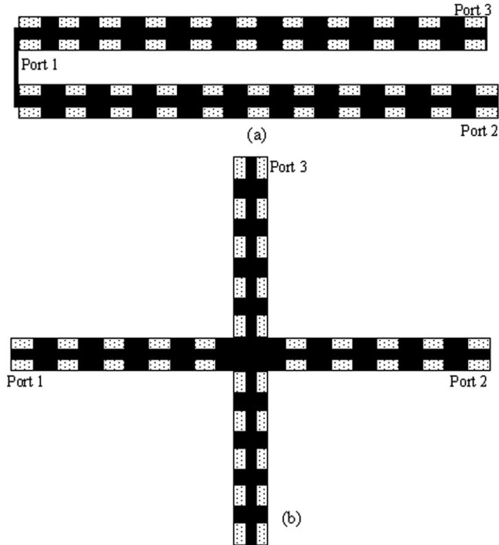
**Figure 5.** (a) The top view of a parallel duplexer. The input power is fed at Port 1 and transmission is observed in Port 2 and Port 3. (b) The top view of the plus-type frequency selective coupler based on defect-induced MBG structure.
