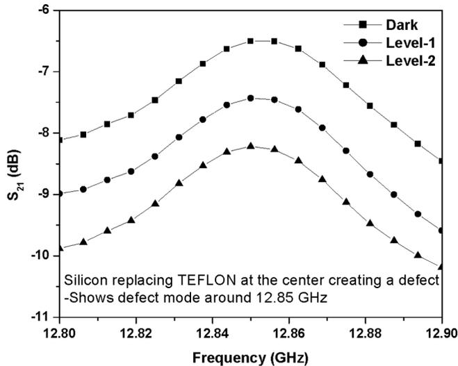
**Figure 4.** The formation of defect mode due to replacement of a PTFE substrate piece with an intrinsic silicon and the variation of transmitted power under photo-excitation.
