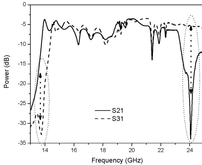
**Figure 6.** Transmission spectra of the parallel duplexor. Lesser transmitted power at Port 3 compared to Port 2 at 13.8 GHz and lesser transmitted power at Port 2 compared to Port 3 at around 24.1 GHz.
