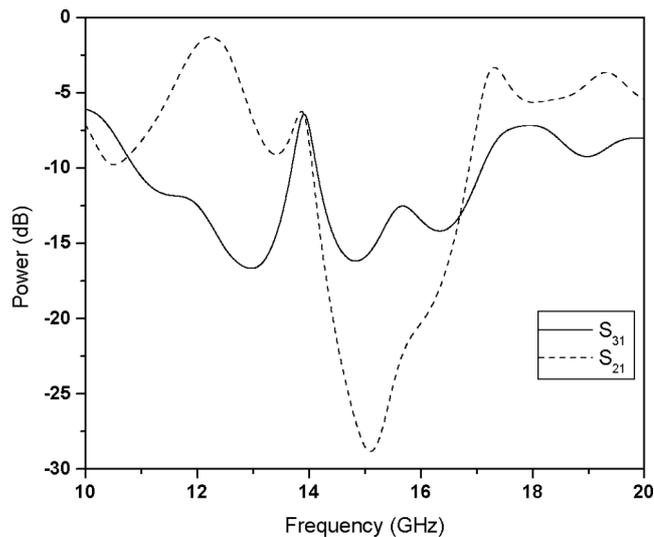
**Figure 7.** The transmission spectra between Ports 1 and 2 and between 1 and 3 for the structure given in figure 5b.
