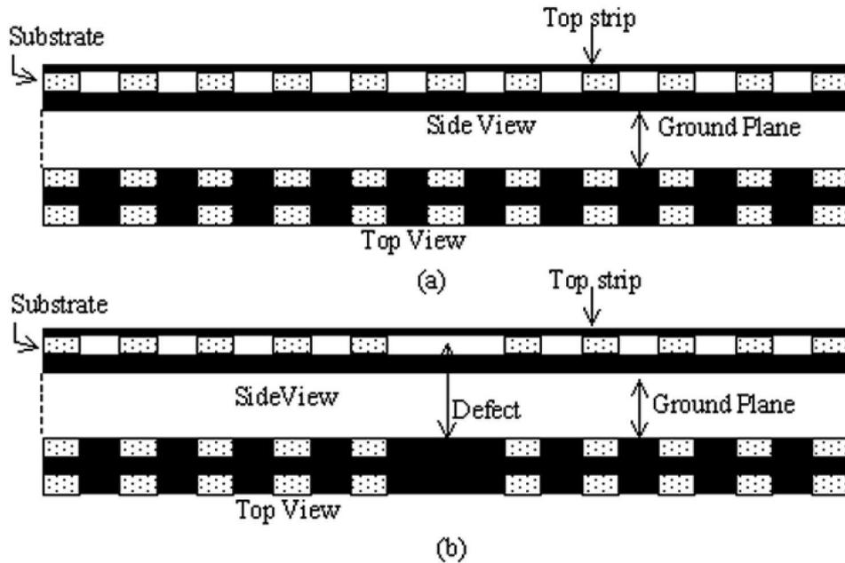
**Figure 1.** The microstrip microwave band gap structure, (a) without a defect and (b) with an acceptor defect.
