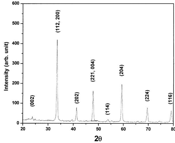
Figure 1. XRD pattern of LCMO sample.
