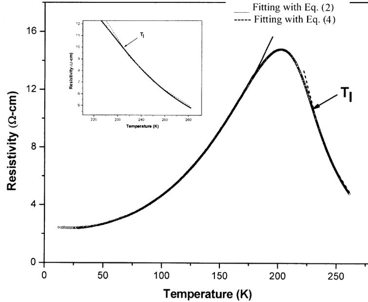
**Figure 3.** Resistance vs. temperature curve with its theoretical fittings by VRH model.
