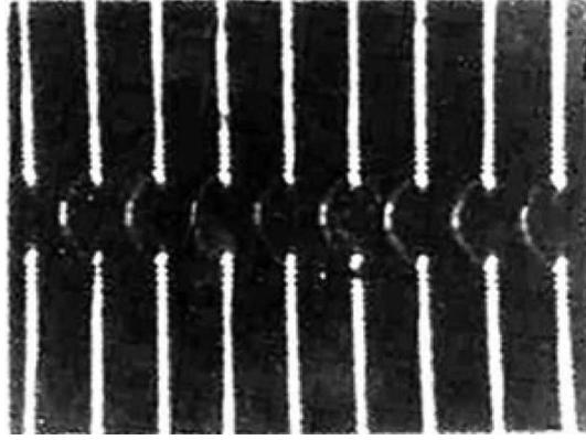
**Figure 2.** Experimental photograph of straight line fringes modulated by the phase shift introduced by the fiber, where  $d = 109.03 \mu\text{m}$  is the fiber diameter,  $\mu_L = 1.5154$  is the liquid refractive index,  $\mu_{\text{fiber}} = 1.5172$  is the fiber refractive index,  $dz/\Delta z = 0.4907$  is the differential fringe shift,  $\lambda = 632.8 \text{ nm}$  is the laser wavelength. Experiment is operated at room temperature  $T = 25.5^\circ\text{C}$ .
