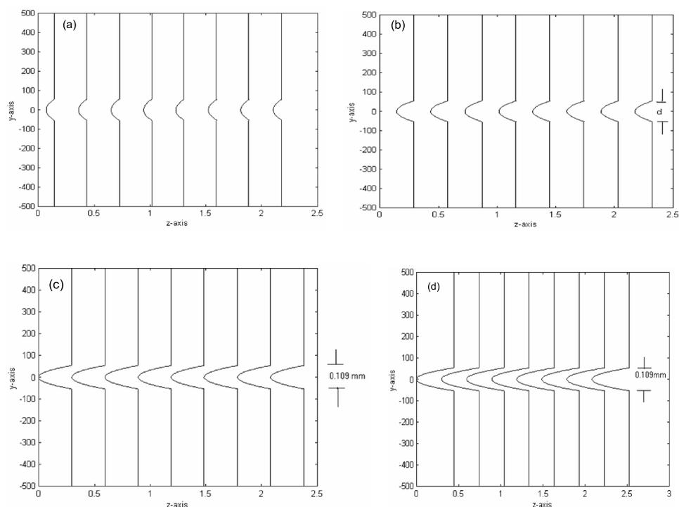
**Figure 3.** Plot of fringes modulated by a parabolic function of full width = 0.109 mm,  $y$ -axis and  $z$ -axis are in micrometric scale and the differential fringe shift is equal to (a) 0.25, (b) 0.5, (c) 1.0 and (d) 1.25.
