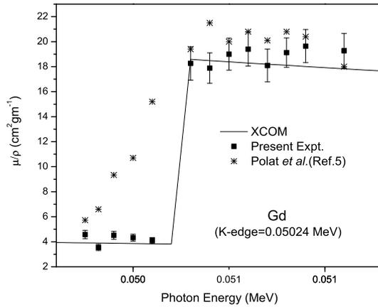
Figure 7. Comparison of the attenuation coefficients for Gd with XCOM values.
