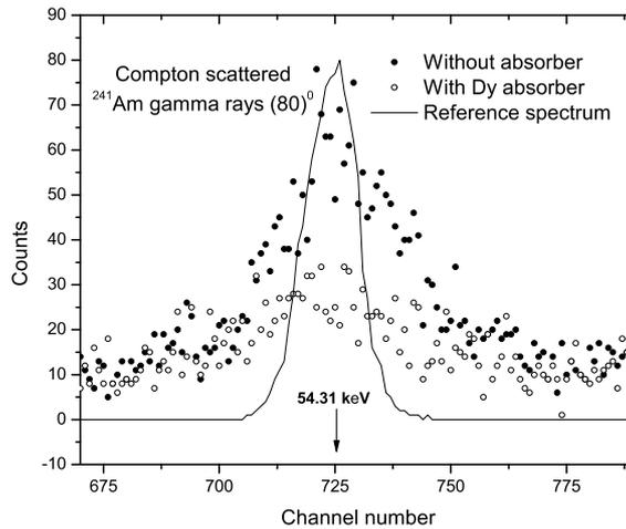
**Figure 2.** Comparison of spectra of Compton scattered radiations from a  $^{241}\text{Am}$  source at  $80^\circ$  with and without the pellet absorber (Dy) with that of monoenergetic gammas of energy 54.31 keV.
