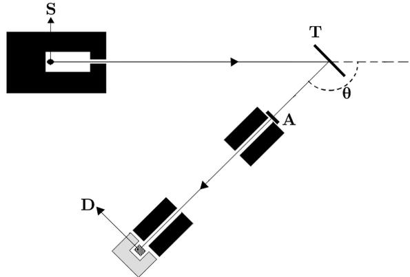
**Figure 1.** Schematic diagram of the experimental set-up for narrow beam geometry gamma attenuation measurements.
