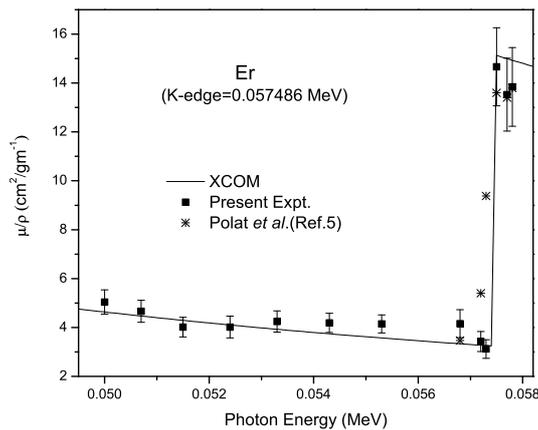
**Figure 9.** Comparison of the attenuation coefficients for Er with XCOM values.
