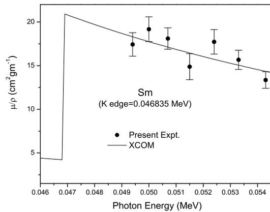
**Figure 5.** Comparison of the attenuation coefficients for Sm with XCOM values.
