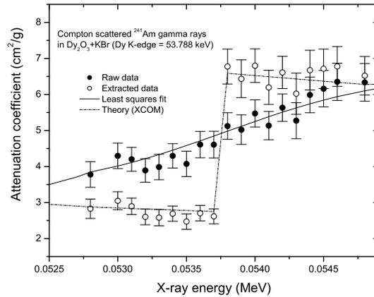
**Figure 3.** Variation of the attenuation coefficient with energy for a mixture of dysprosium oxide and potassium bromide.
