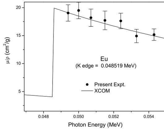
Figure 6. Comparison of the attenuation coefficients for Eu with XCOM values.
