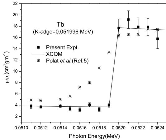
**Figure 8.** Comparison of the attenuation coefficients for Tb with XCOM values.
