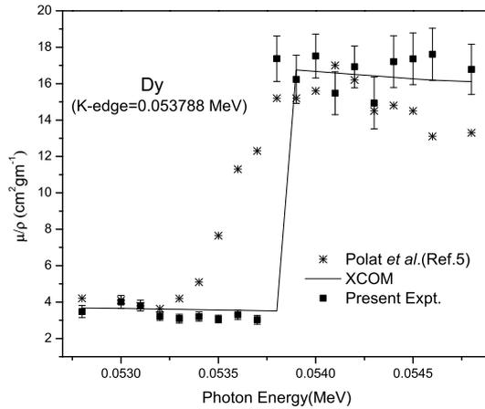
**Figure 4.** Comparison of the attenuation coefficients for Dy with XCOM values.
