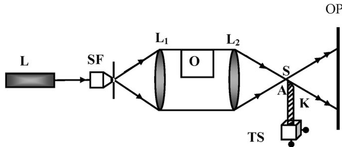
**Figure 1.** Schematic experimental setup of Schlieren diffraction interferometer.
