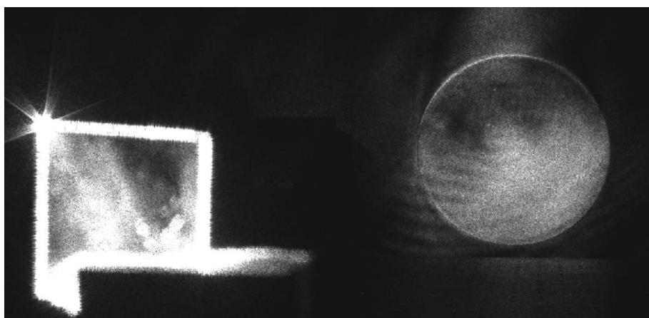
**Figure 2.** Square phase aperture with its corner illuminated with a focused laser beam (left) and corresponding infinite mode diffraction pattern (right).
