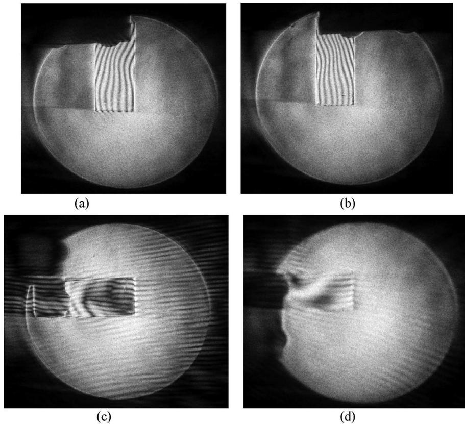
**Figure 4.** Test results of an optical glass plate with phase knife-edge as Schlieren diffracting element.
