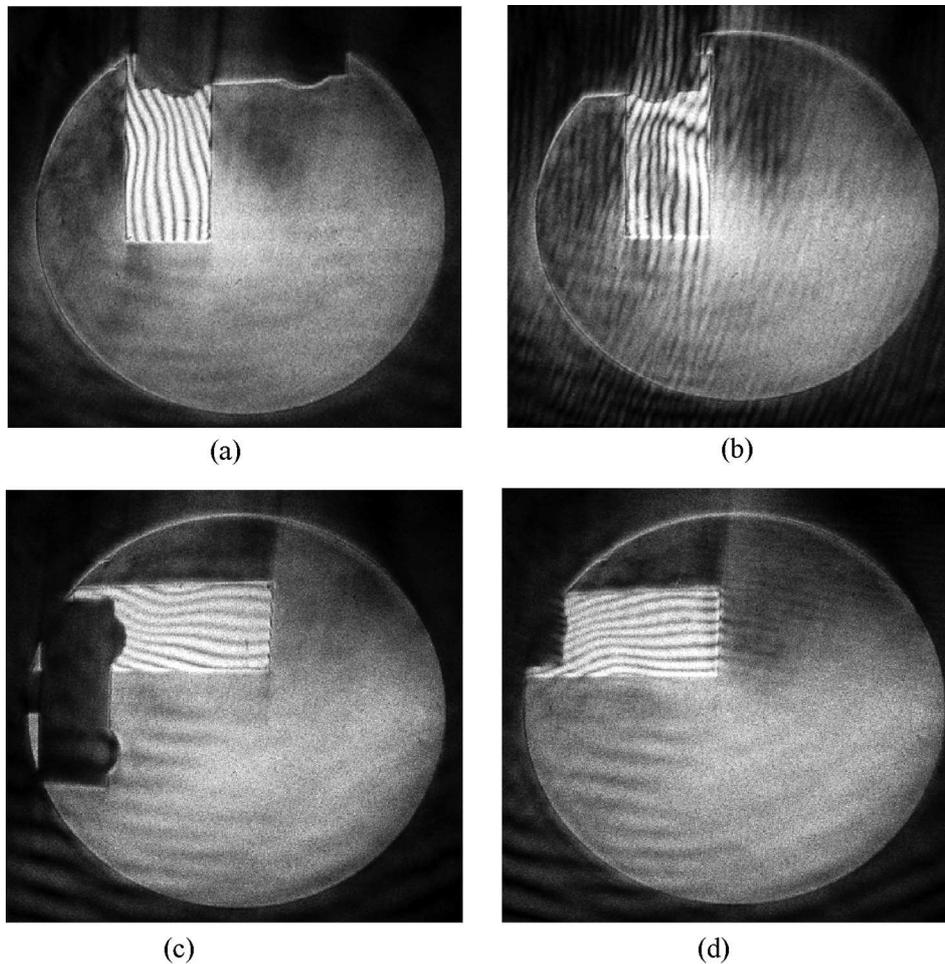
**Figure 3.** Test results of an optical glass plate with corner of a square phase aperture as Schlieren diffracting element.
