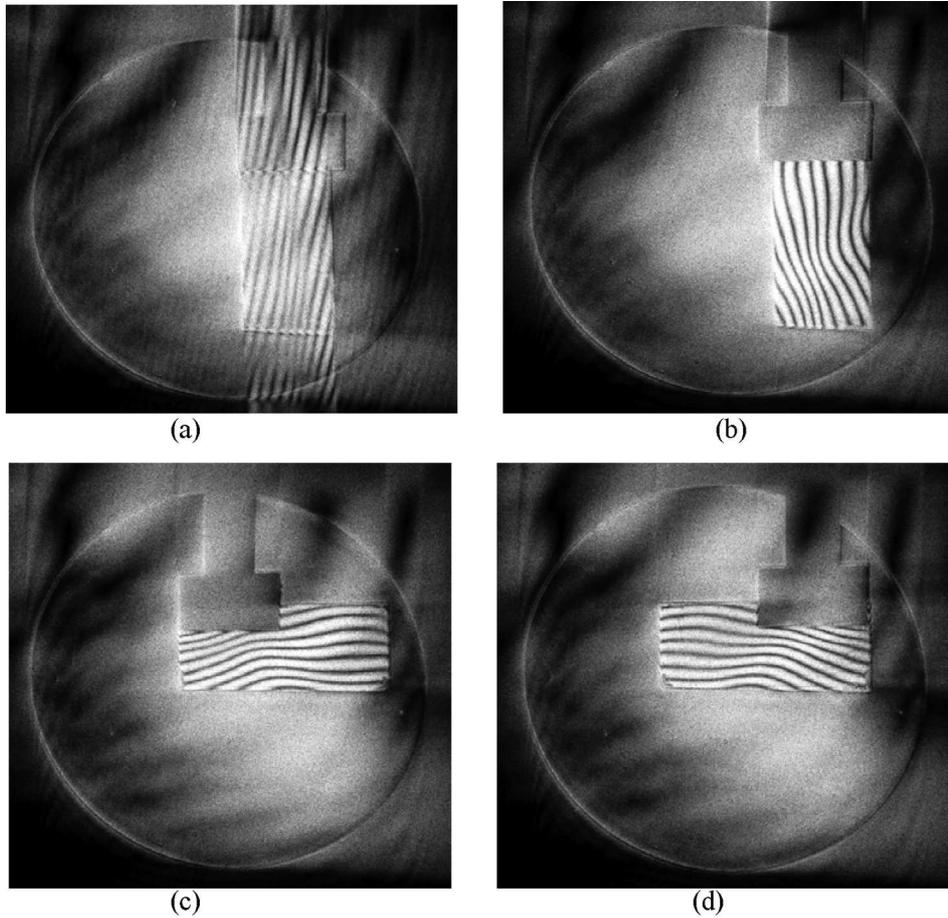
**Figure 5.** Test results of an optical glass plate with an optical fiber tip as Schlieren diffracting element.
