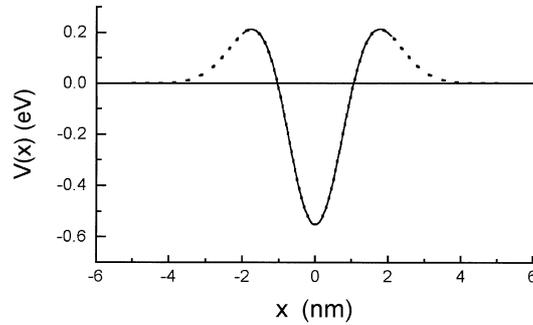
**Figure 7.** Plot of potential given by (23) as a function of distance with values of parameter  $J = 0.55$  eV and  $\lambda = 0.5$ . The full potential is shown as dashed curve where the part covering the well region is marked by solid curve.
