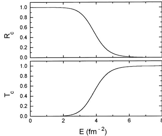
**Figure 3.** Comparison of reflection  $R_c$  and transmission  $T_c$  coefficients as a function of energy given by expressions (10) and (11), respectively, with the corresponding results obtained from expressions (14) and (15).
