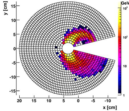
**Figure 4.** Energy flux from beamstrahlung pairs at the BeamCal  $z$ -position for a 20 mrad and DID field configuration (LDC coordinate system). An angular range of  $40^\circ$  is not instrumented in the region of the incoming beam.
