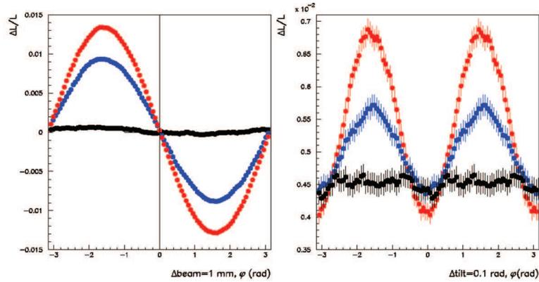
**Figure 3.** Relative shift in the luminosity as a function of the azimuthal angle of a beam offset of 1 mm (left) and of the azimuthal angle of a polar tilt angle of 0.1 rad (right). The cases are: LumiCal centered along the outgoing beam (black) and centered on the detector axis for a 14 mrad (blue) or 20 mrad (red) crossing angle [4].
