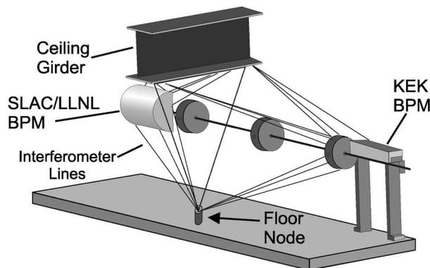
**Figure 1.** Arrangement of a proposed ATF network, for monitoring relative movement between two sets of beam position monitors (BPM)s. The axial line between the BPMs represents the beam pipe.
