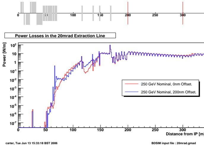
**Figure 1.** Normalised power losses along the 20 mrad extraction line from disrupted beam and SR. Total integrated power of 1.68 W (1.66 W) for 0 nm (200 nm) vertical offset.
