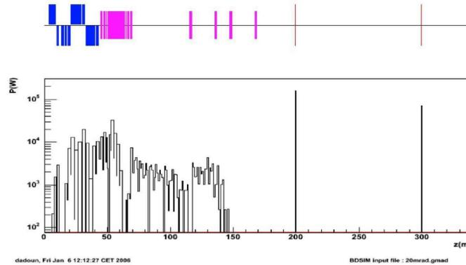
**Figure 4.** Power loss along the 20 mrad extraction line for the high luminosity 1 TeV, 80 nm vertical offset beam.
