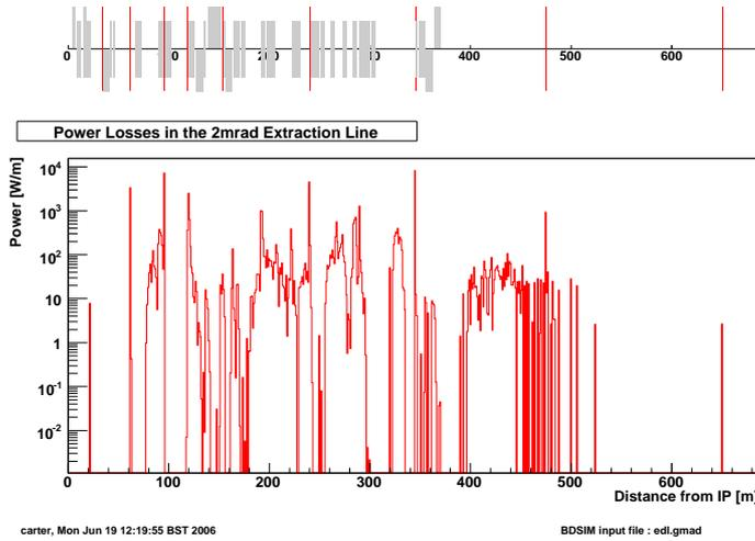
**Figure 2.** Normalised power losses along the 2 mrad extraction line for 250 GeV nominal disrupted beam with SR but no vertical offset. Total integrated power of 45.8 kW.
