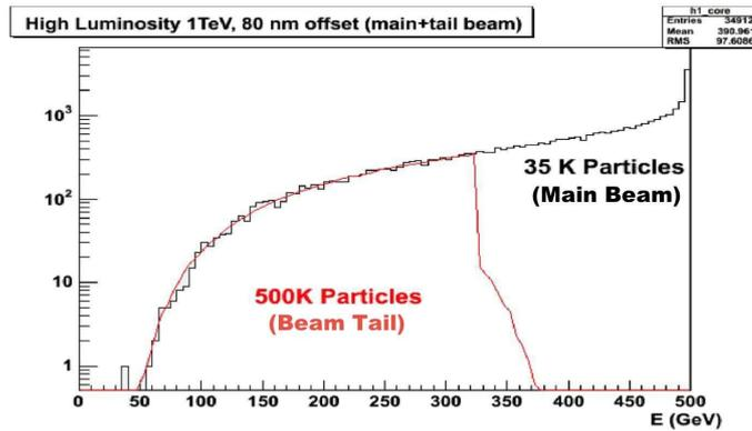
**Figure 3.** Energy spectrum for the high luminosity 1 TeV, 80 nm vertical offset, disrupted beam.
