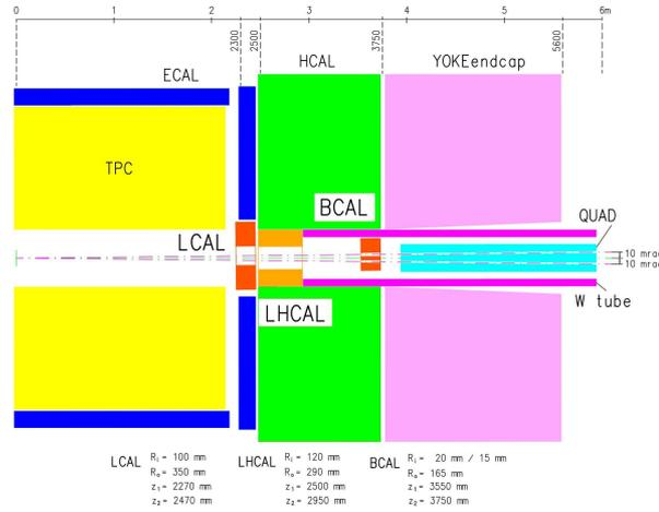
**Figure 1.** Forward region of the LDC detector for a 20 mrad crossing angle. TPC: time projection chamber, ECAL: electromagnetic calorimeter, HCAL: hadronic calorimeter, LCAL: luminosity calorimeter, LHCAL: low angle hadronic calorimeter, BCAL: beam calorimeter. The LCAL and BCAL are centred around the outgoing beam.
