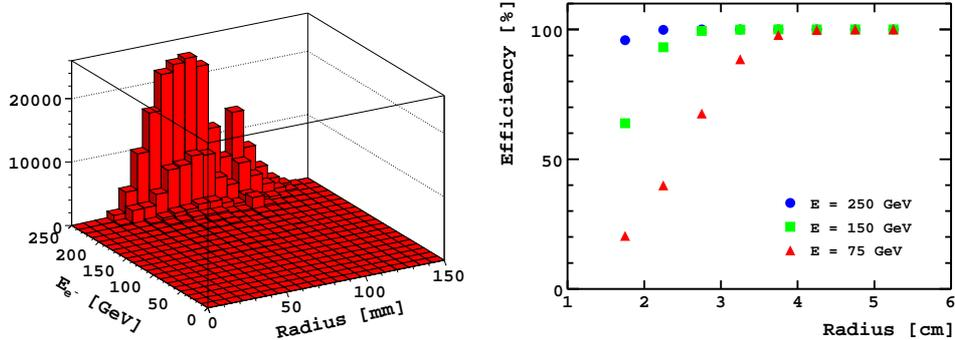
**Figure 2.** Left: Electron energy and spatial distribution of the two-photon background events passed all selection cuts except the BeamCal veto. Right: The efficiency to veto an electron of energy 75, 150, 250 GeV as a function of the radius in the BeamCal.
