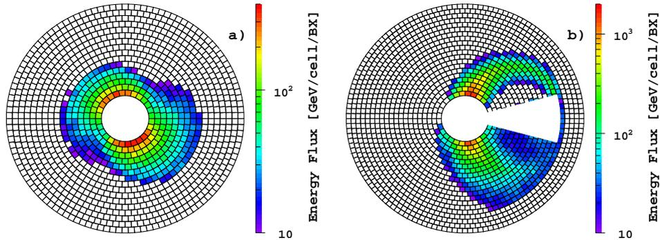
**Figure 1.** The energy density of beamstrahlung remnants per bunch crossing as a function of position in the  $r$ - $\varphi$  plane at (a) 2 mrad and (b) 20 mrad with DID field crossing angles.
