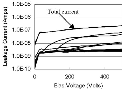
**Figure 1.** *IV* characteristics of the 32 strips of the strip detector.
