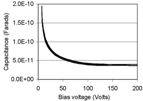
**Figure 2.** *CV* characteristics of all the 32 strips of the strip detector.
