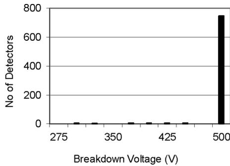
**Figure 3.** Distribution of the breakdown voltage for 800 detectors.
