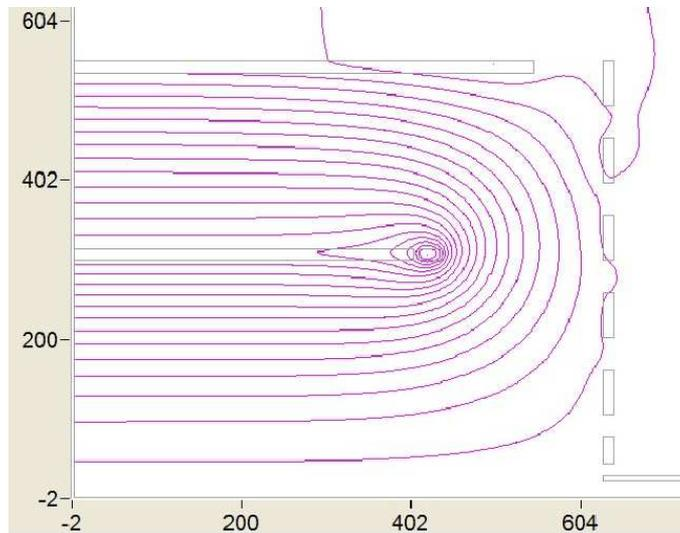
**Figure 1.** The magnetic field of the 4th concept showing the dual solenoids and the circular coils closing off the end cap regions by redirecting the magnetic field into the return annulus.
