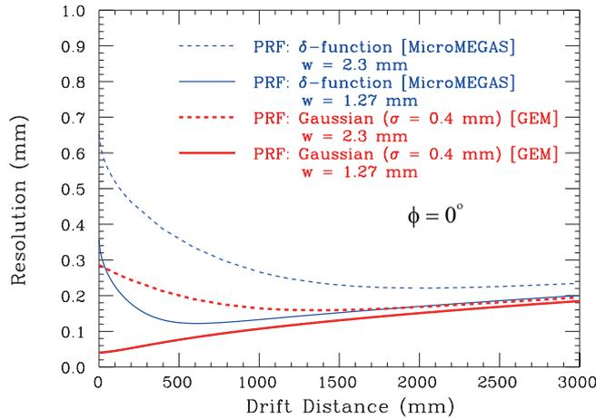
**Figure 4.** Expected spatial resolutions of the ILC-TPC obtained with MicroMEGAS or GEMs. Gas: Ar-methane (5%),  $E = 100$  V/cm,  $B = 4$  T ( $D = 50 \mu\text{m}/\sqrt{\text{cm}}$ ), and  $N_{\text{eff}} = 22$ .
