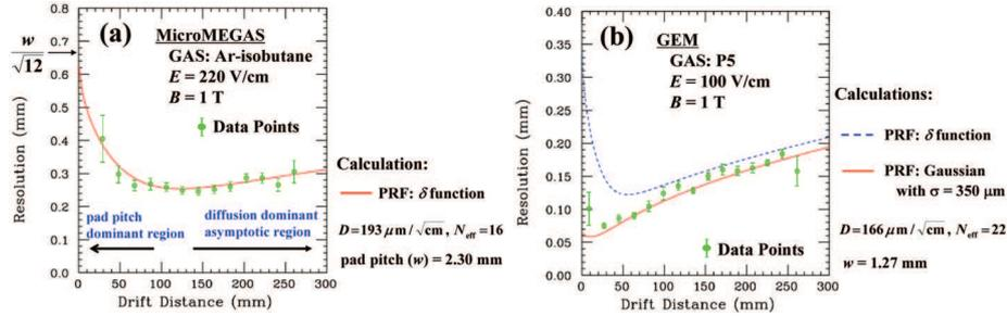
**Figure 3.** (a) Spatial resolution vs.  $z$  obtained with MicroMEGAS,  $w = 2.3$  mm, gas: Ar–isobutane (5%). (b) Spatial resolution vs.  $z$  obtained with GEMs,  $w = 1.27$  mm, gas: Ar–methane (5%).
