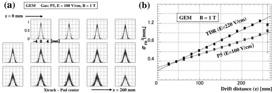
**Figure 2.** (a) Pad responses for different drift distances. (b) Pad response width squared ( $\sigma_{PR}^2$ ) vs. drift distance ( $z$ ). The width of pad response is parametrized as  $\sigma_{PR}^2 = \sigma_{PR0}^2 + D^2 \cdot z$ , with  $D$  being the diffusion constant.
