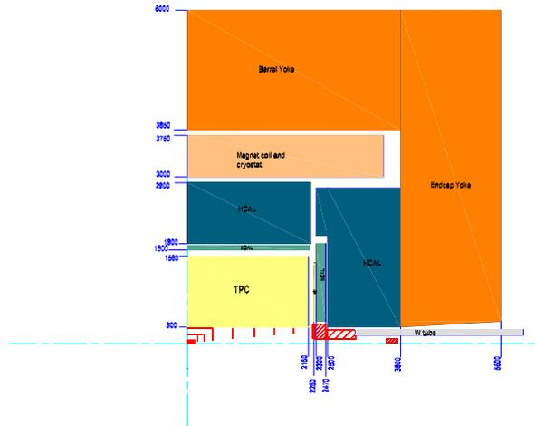
**Figure 1.** Side-view of the LDC detector concept.
