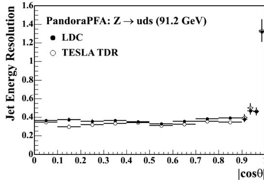
**Figure 3.** Simulated resolution of the LDC detector concept as a function of  $\cos(\theta)$ , using a particle flow approach.
