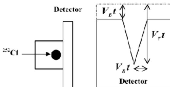
**Figure 1.** A schematic diagram showing the experimental arrangement and determination of bulk and track etch rates.
