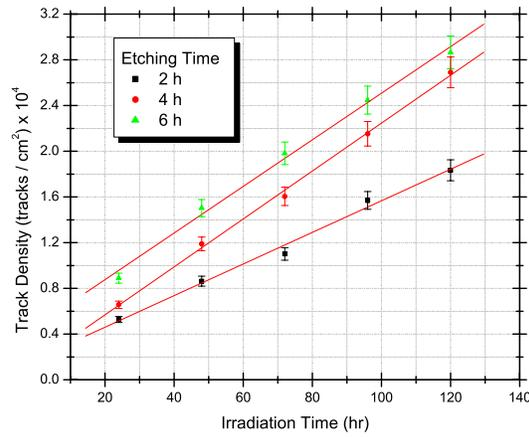
**Figure 2.** The dependence of the track density on the irradiation time in CR-39 plastic detector.
