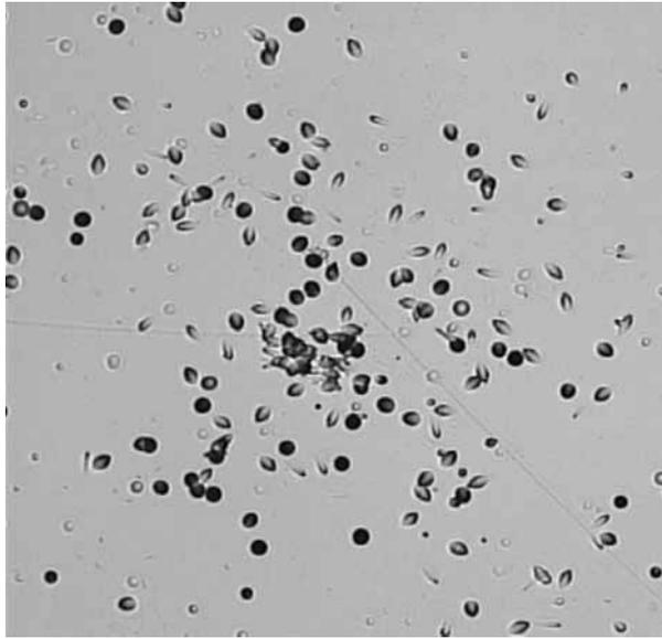
**Figure 4.** Photomicrograph of recoil tracks in CR-39 plastic detector irradiated with  $^{252}\text{Cf}$  neutron source, etched in 6.25 N NaOH at  $70^\circ\text{C}$  for 4 h at magnification  $600\times$ .
