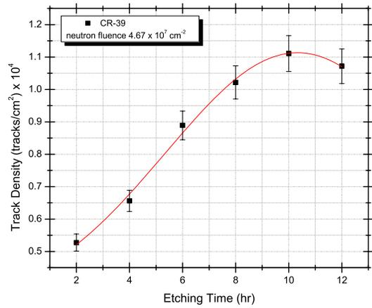
**Figure 3.** The variation of track density as a function of etching time for CR-39 detector.
