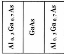
**Figure 1.** Schematic diagram of a QW formed by stacking a semiconductor (GaAs) sandwiched between the layers of other semiconductor ( $\text{Al}_{0.3}\text{Ga}_{0.7}\text{As}$ ).
