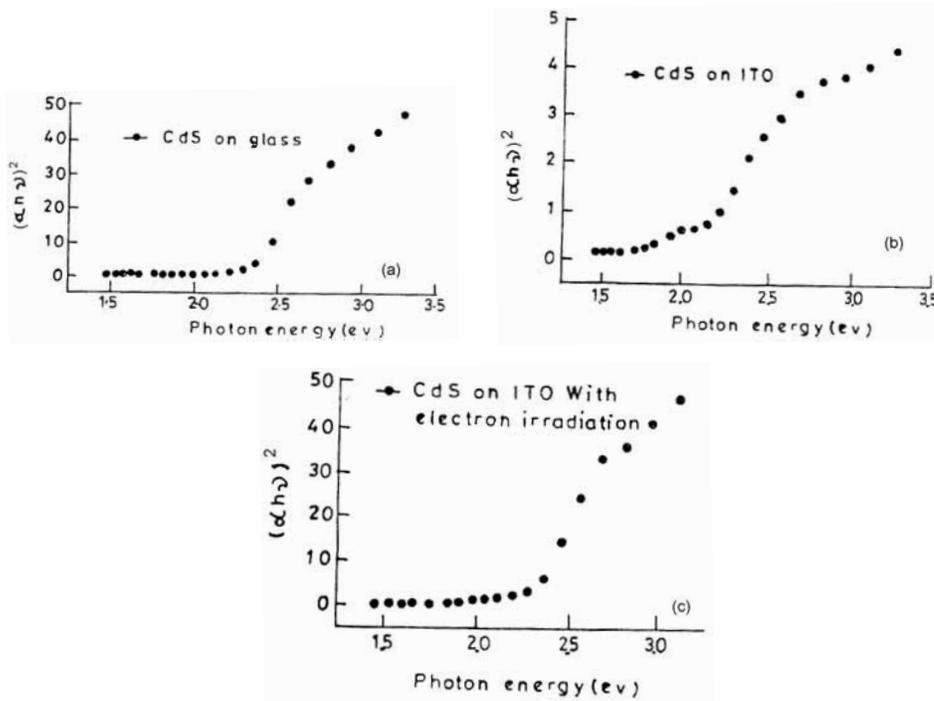
**Figure 2.** The graph showing photon energy (eV) vs.  $(\alpha h\nu)^2$  for CdS thin films. (a) CdS film on glass, (b) CdS film on ITO conducting surface, (c) CdS film on ITO conducting surface with electron irradiation.
