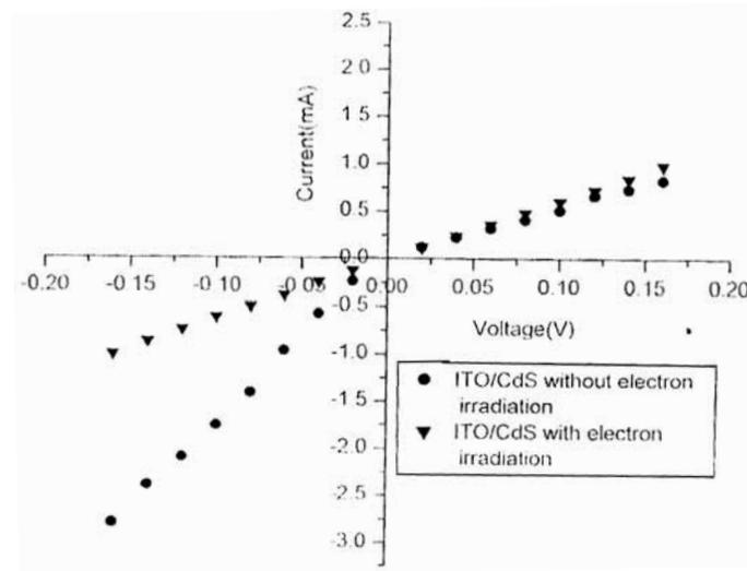
**Figure 3.** The  $V-I$  characteristics of ITO/CdS film with and without electron irradiation.
