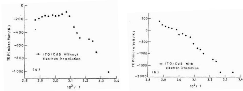
**Figure 5.** The thermoelectric power vs.  $10^3/T$ . (a) ITO/CdS without electron irradiation, (b) ITO/CdS with electron irradiation.
