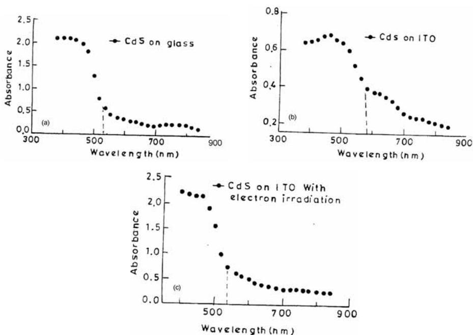
**Figure 1.** Absorbance spectra of CdS thin films with photon wavelength. (a) CdS film on glass, (b) CdS film on ITO conducting surface, (c) CdS film on ITO conducting surface with electron irradiation.
