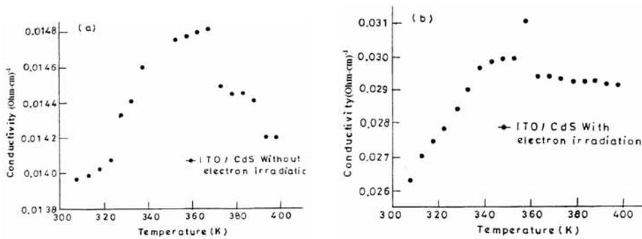
**Figure 4.** The conductivity vs. temperature. (a) ITO/CdS without electron irradiation, (b) ITO/CdS with electron irradiation.
