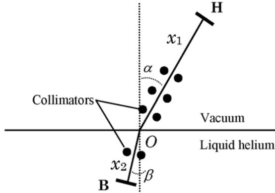
**Figure 1.** Co-positions of the heater H and the bolometer B. Here the angle  $\alpha$  between the heater H and the liquid surface normal is  $30^\circ$  and the distance  $x_1$  is  $\sim 25$  mm. The angle  $\beta$  between the bolometer B and the normal is  $10^\circ$  and the distance  $x_2$  is  $\sim 7$  mm.
