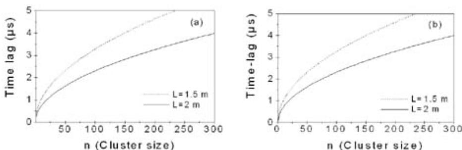
**Figure 5.** Time-lag changes with the cluster sizes  $n$ . (a) Beam source parallel to the spectrometer axis and (b) beam source perpendicular to the axis.
