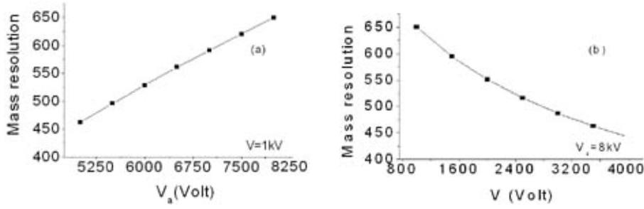
**Figure 3.** Mass resolution vs. voltage variation. (a)  $V_a$  is varied and  $V$  kept constant, (b)  $V$  is varied and  $V_a$  kept constant.
