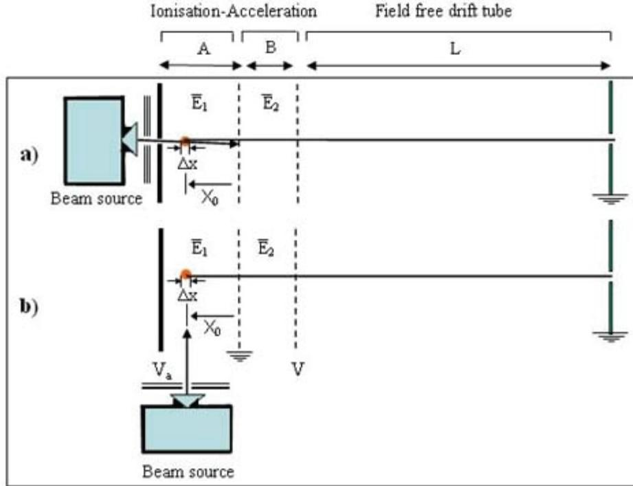
**Figure 1.** Block diagram of the ToF spectrometer. (a) Spectrometer with the cluster beam source along the axis. (b) Spectrometer with the cluster beam source perpendicular to the axis.
