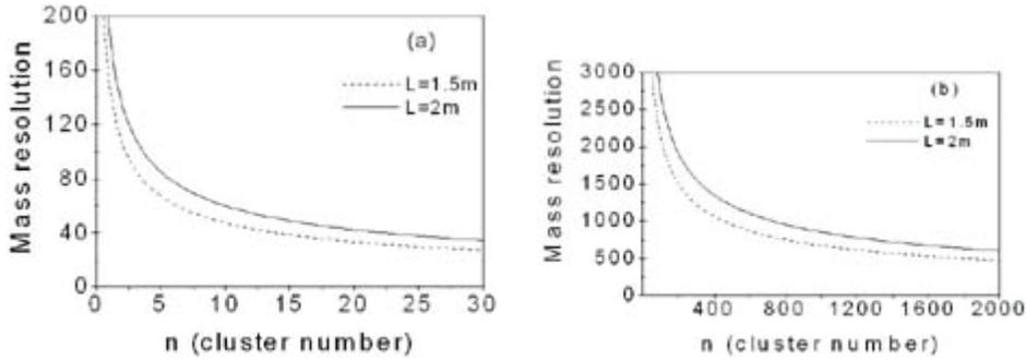
**Figure 2.** Mass resolution variation with the cluster size  $n$ . (a) Beam source parallel to the spectrometer axis and (b) beam source perpendicular to the axis.
