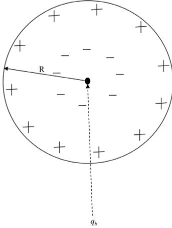
**Figure 1.** Schematic diagram showing a test charge  $q_b$  (assumed positive) inserted at the centre of a spherical quasi-neutral plasma. The accumulation of induced negative charges around the centre and positive charges at the surface layer are marked.
