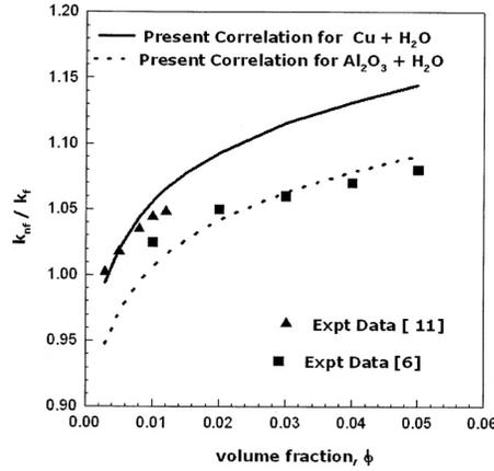
**Figure 2.** Comparison of the present correlation with the experimental data [6,11].
