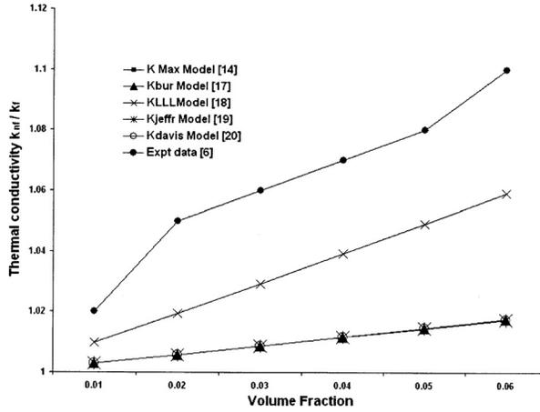
**Figure 1.** Comparison of the thermal conductivity of nanofluid models with the experimental data [6].
