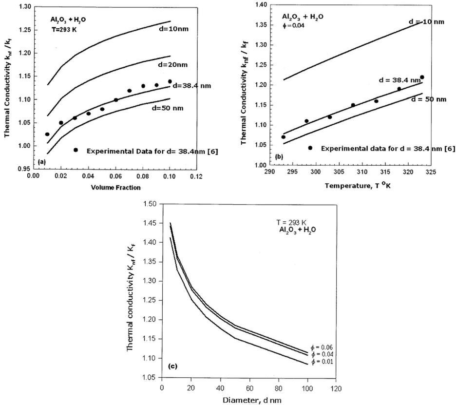
Figure 3. The effect of (a) volume fraction, (b) temperature and (c) diameter of nanoparticle on thermal conductivity of nanofluid.
