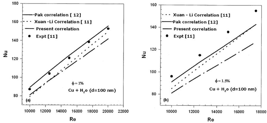
**Figure 5.** Nusselt number comparison for Cu + water nanofluid correlation with the experimental data. (a)  $\phi = 1\%$ , (b)  $\phi = 1.5\%$ .
