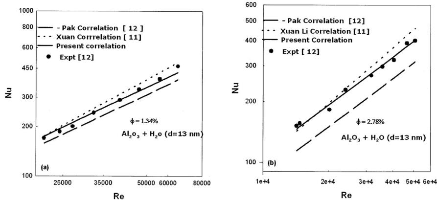
**Figure 4.** Nusselt number comparison for alumina + water nanofluid correlation with the experimental data. (a)  $\phi = 1.34\%$ , (b)  $\phi = 2.78\%$ .
