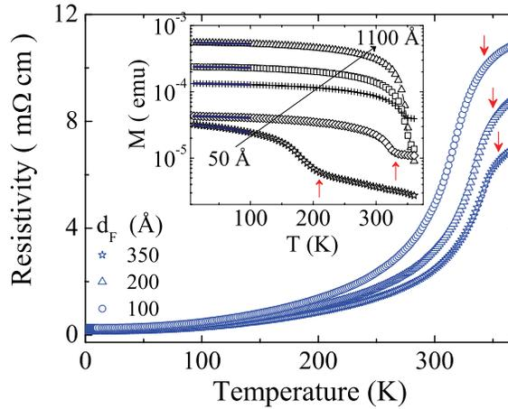
**Figure 1.** Resistivity ( $\rho(T)$ ) of LSMO films deposited on STO in the temperature range of 2–370 K. Thickness of the films varies from 100 Å to 350 Å. Inset: The 1000 Oe field-cooled magnetization of single layer LSMO films of thickness ranges from 50 Å to 1100 Å. In all cases the magnetic field was applied in the plane of the film. The solid lines are fits to the Bloch relation (see text for details). Curie temperatures have been marked by the arrows.
