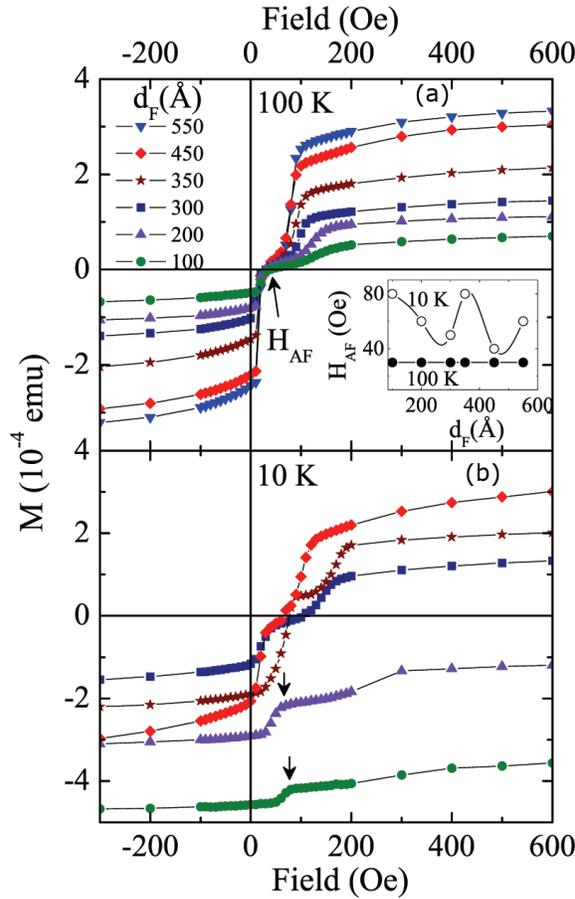
**Figure 4.** Panels (a) and (b) show the last two quadrants of zero-field-cooled hysteresis curves at 100 K and 10 K respectively. All measurements were carried out with a field-in-plane geometry. The inset in panel (a) compares the antiferromagnetic coupling field  $H_{AF}$  (indicated by arrows in some cases) at temperatures 10 K and 100 K, as a function of the thickness of LSMO boundary ( $d_F$ ). The solid lines in the inset are only guides to the eyes.
