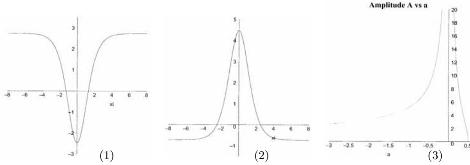
**Figure 2.** (1) Dark soliton of eq. (1) for  $a=1, b=-1, d_1=-1, c=1$ ; (2) Bright soliton of eq. (1) for  $a=1, b=1, d_1=-1, c=1$ ; (3) Plot of amplitude  $A$  vs  $a$  for  $d_1=1, c=1$ .
