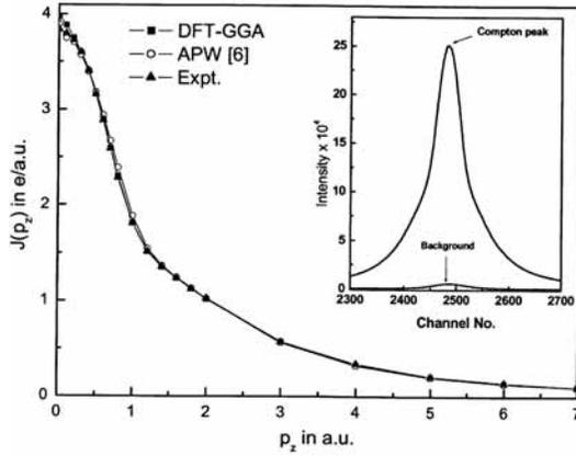
**Figure 4.** Duly corrected isotropic experimental Compton profile of test sample Al along with convoluted APW theory [6] and the present DFT-GGA profiles. The experimental errors are within the size of symbols used. In the inset, the raw data of Al along with the background are shown. Each data is for a period of 21.22 h.
