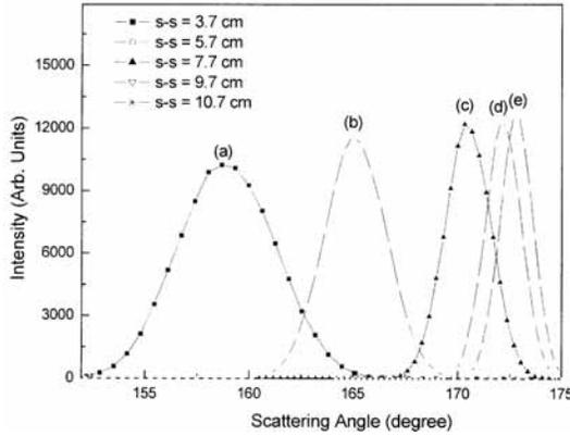
**Figure 2.** Monte Carlo-based geometrical divergence for typical distances between source and sample (s-s) as detailed in table 1. The present spectrometer is based on the geometrical divergence produced by the peak (b).
