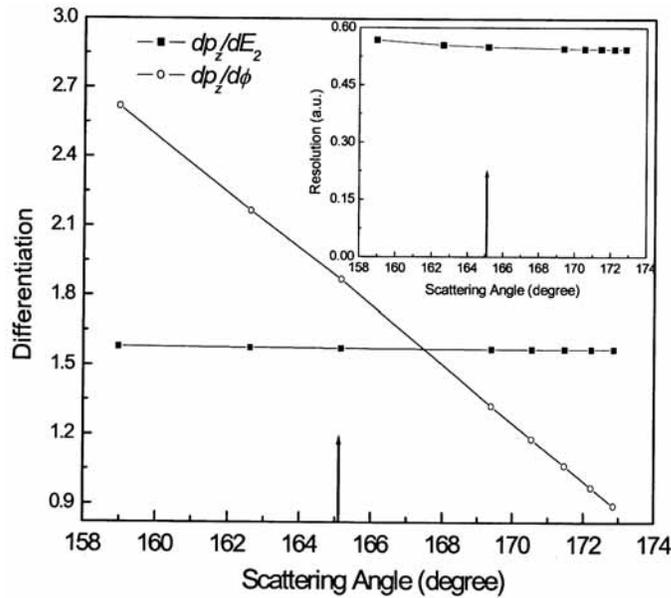
**Figure 3.** Plot of  $dp_z/dE_2$  (a.u./keV) and  $dp_z/d\phi$  (a.u./rad.) for different angles. In the inset, overall momentum resolution (computed using eq. (4)) is also shown. Detector resolution,  $\Delta E_2$ , in the present set-up is 346 eV at 48.4 keV. The vertical arrow shows the scattering angle chosen in the present set-up.
