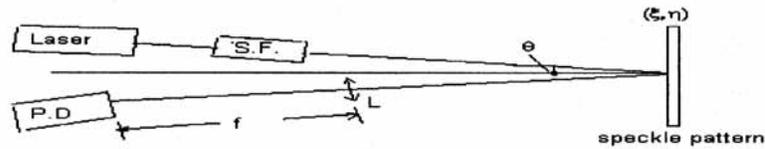
**Figure 3.** Recording of the autocorrelation function at the plane  $(x', y')$  conjugate to the rough object plane  $g(x, y)$  from the speckle pattern situated in the plane  $(\xi, \eta)$ . SF: spatial filter; L: lens of focal length  $f = 15$  cm.
