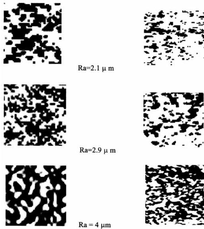
**Figure 2.** Detection of speckle images (left) and the corresponding autocorrelation images (right) for different surfaces of aluminum using CCD camera.
