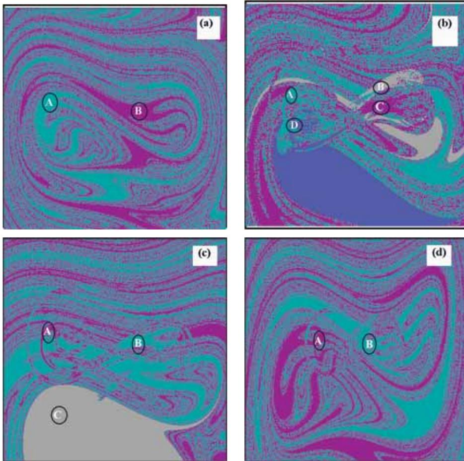
**Figure 4.** The basin structures for the coupled double-well Duffing oscillators for different values of the coupling strength. The parameters are:  $g = 0.095, b = 0.1$  and  $\omega = 0.88$ . (a)  $k = 0$ , (b)  $k = 0.25$ , (c)  $k = 0.8$ , (d)  $k = 1.5$ . The  $x$  and  $y$  variables are plotted in the oscillator 1 coordinates in the range  $-2.0 \leq x, y \leq 2.0$ .
