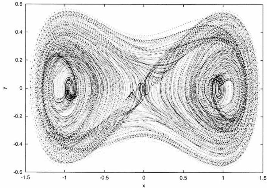
**Figure 1.** Cross-well chaotic attractor in the  $x, y$  ( $y = \dot{x}$ ) plane for  $b = 0.1, g = 0.095$  and  $\omega = 0.79$ .
