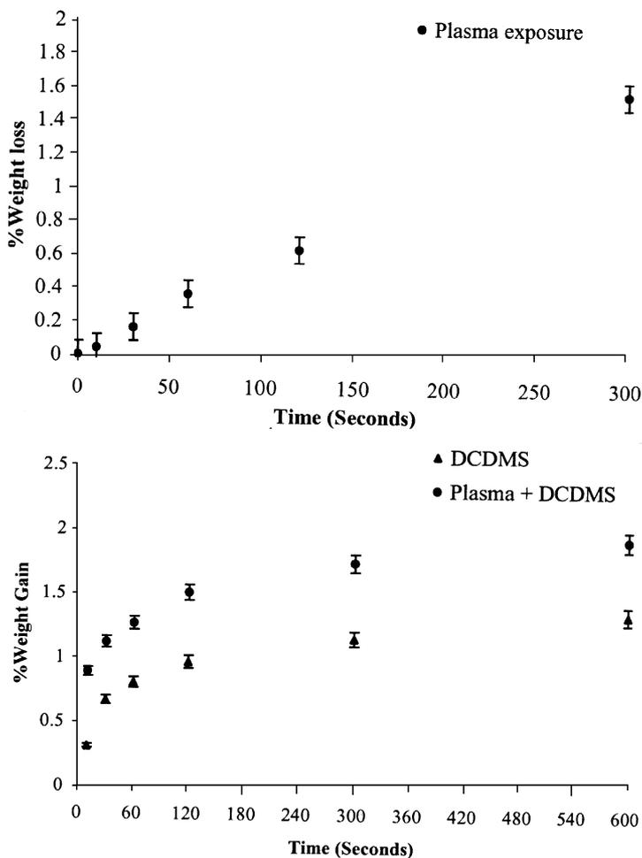
Figure 1. (a) Percentage weight loss of polyester fabric after plasma treatment. (b) Percentage weight change of polyester fabric treated with DCDMS.
