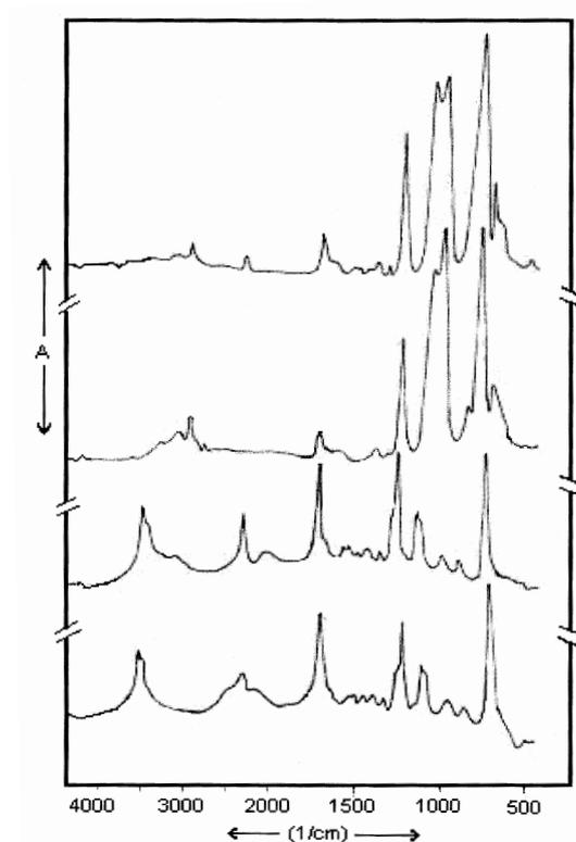
**Figure 4.** IR spectra of polyester fabric, (a) untreated; (b) 2-min plasma exposed; (c) 2-min DCDMS treated and (d) 2-min DCDMS treated after exposure of plasma for 2 min.
