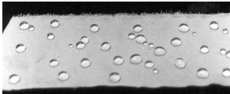
**Figure 3.** Photograph of 10-s DCDMS treated polyester fabric.
