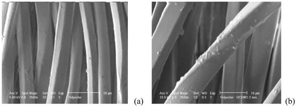
**Figure 2.** SEM micrograph of (a) untreated polyester fabric and (b) 2-min DCDMS treated polyester fabric.
