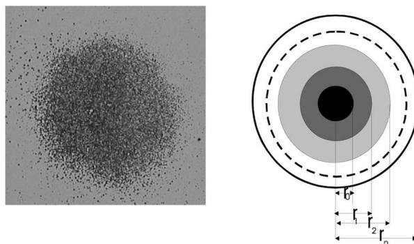
**Figure 8.** Photo of an individual microbeam (left) and schematic diagram of the equivalent CCZ model (right).
