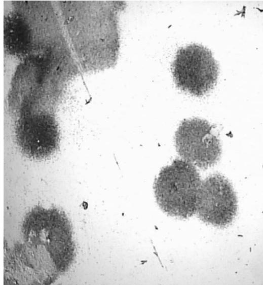
**Figure 3.** Photo of a collection of microbeams of plasma ion tracks developed by chemical etching.
