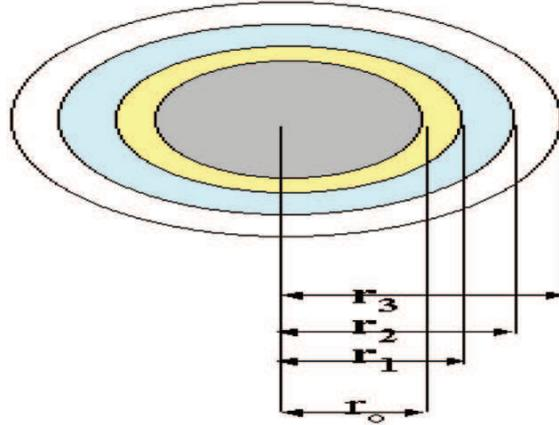
**Figure 2.** Schematic diagram of the CCZ model, where  $r_0$  is the radius of the core,  $r_1$ ,  $r_2$  and  $r_3$  are the radii of the first, second and third zones, respectively.
