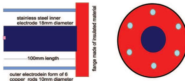
**Figure 1.** Schematic diagram of the construction details of plasma focus electrodes set-up. Left part shows the horizontal cross-section, while the right part shows the vertical cross-section.
