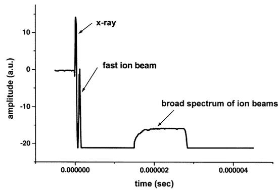
**Figure 7.** Typical Faraday cup signal obtained from a single discharge.
