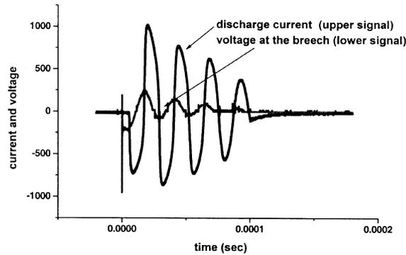
**Figure 4.** Discharge current and voltage signals from the plasma device.
