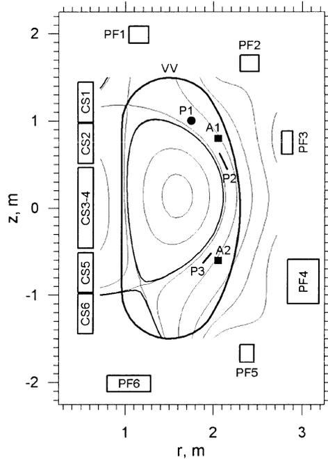
**Figure 1.** Cross-section of the plasma and locations of passive structure consisting of the vacuum vessel (VV) and passive stabilizers (P1, P2, P3). A1, A2 are active feedback coils, CS1–CS6 are central solenoid coils and PF1–PF6 are poloidal field coils.
