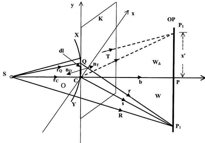
**Figure 1.** Diffraction geometry of the phase knife-edge. XY is a spherical wave-front incident on the phase knife-edge K, T and O denote the phase part and open part in the  $x$ - $y$  plane and C is a point situated on the illuminated boundary of K.
