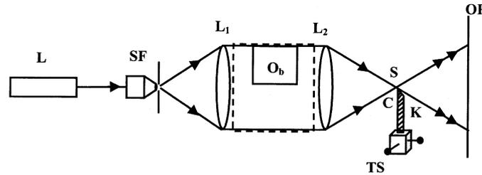
**Figure 2.** Schematic configuration of Schlieren diffraction interferometer.
