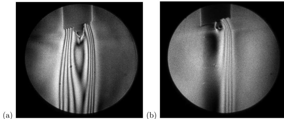
**Figure 4.** Photograph of typical interference pattern of a burning candle in infinite fringe mode (a) with phase knife-edge and (b) with solid knife-edge.
