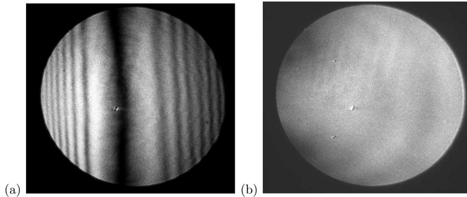
**Figure 3.** Photograph of typical diffraction pattern of phase knife-edge. (a) Finite fringe mode, (b) infinite fringe mode.
