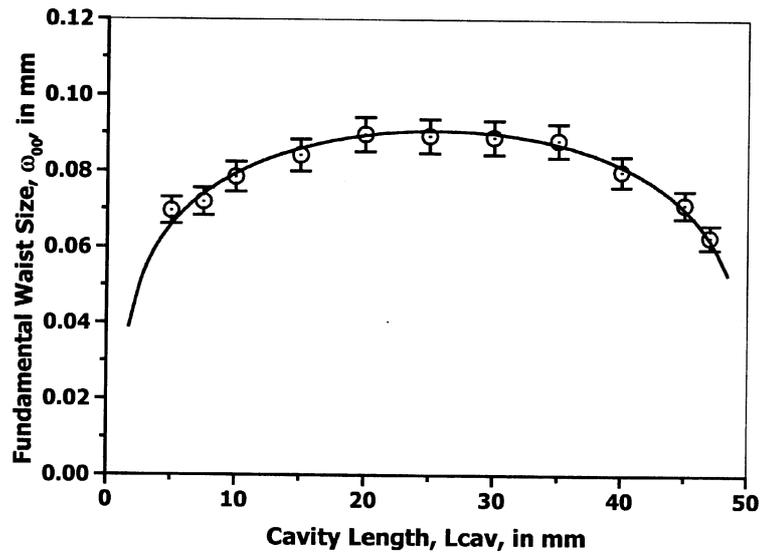
Figure 3. The variation of the fundamental cavity waist size,  $\omega_0$ , with the cavity length,  $L_{cav}$  for a plano-concave cavity.
