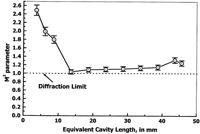
Figure 2. The variation of the beam quality factor,  $M^2$ , as a function of cavity length.
