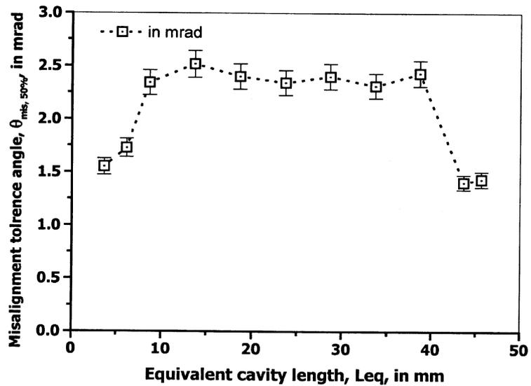
Figure 5. Variation of the misalignment tolerance measured as a function of the cavity length.
