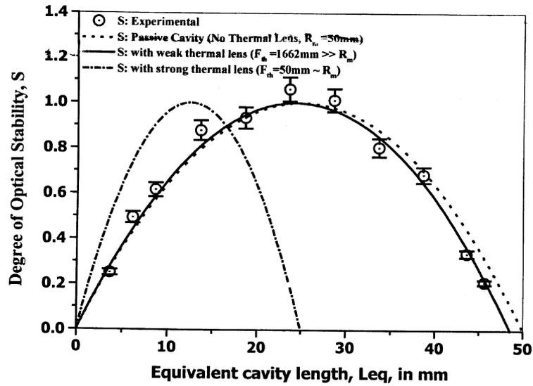
Figure 4. Variation of the degree of optical stability or the  $S$  parameter for a passive and active cavity. *Case 1.* The ROC of the mirror was 50 mm and the wavelength used was  $\lambda_0 = 1064$  nm. *Case 2.* The active cavity  $S$  parameter is plotted in the weak thermal lens limit ( $F_{th} = 1662$  mm). *Case 3.* Strong thermal lens limit ( $F_{th} = R_m = 50$  mm). The measured value of the  $S$  parameter is also plotted.
