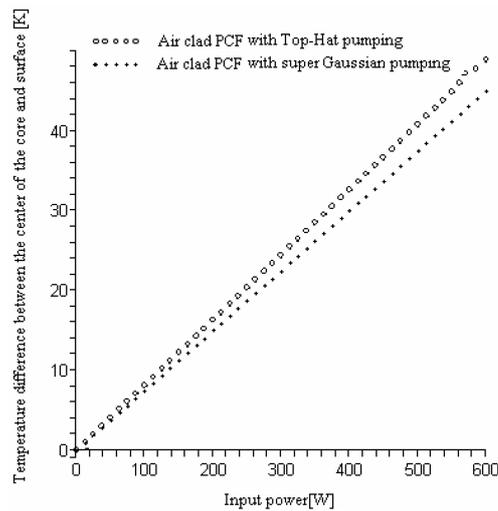
**Figure 3.** Temperature difference between the center of the core and the surface of the PCF laser for both top-hat and super-Gaussian pumping.
