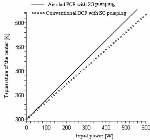
**Figure 2.** Temperature of the center of DCF laser compared to PCF laser as a function of input power.
