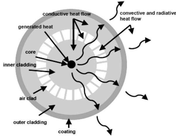
**Figure 1.** Heat flow in air-clad photonic crystal fiber lasers [9].
