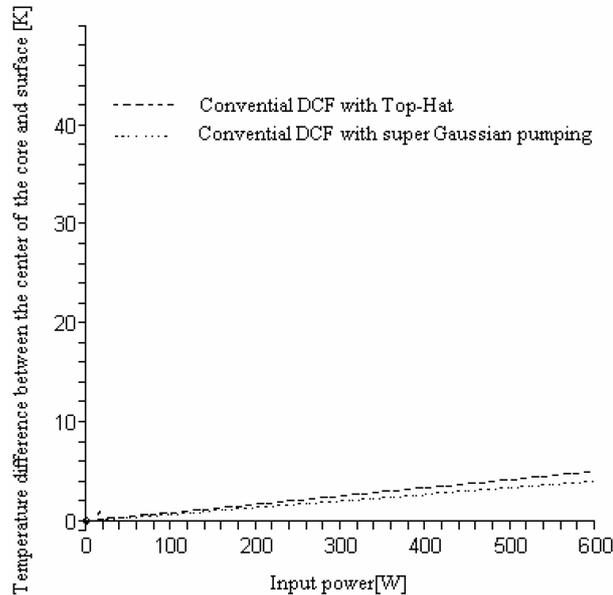
**Figure 4.** Temperature difference between the center of the core and the surface of the DCF laser for both top-hat and super-Gaussian pumping.
