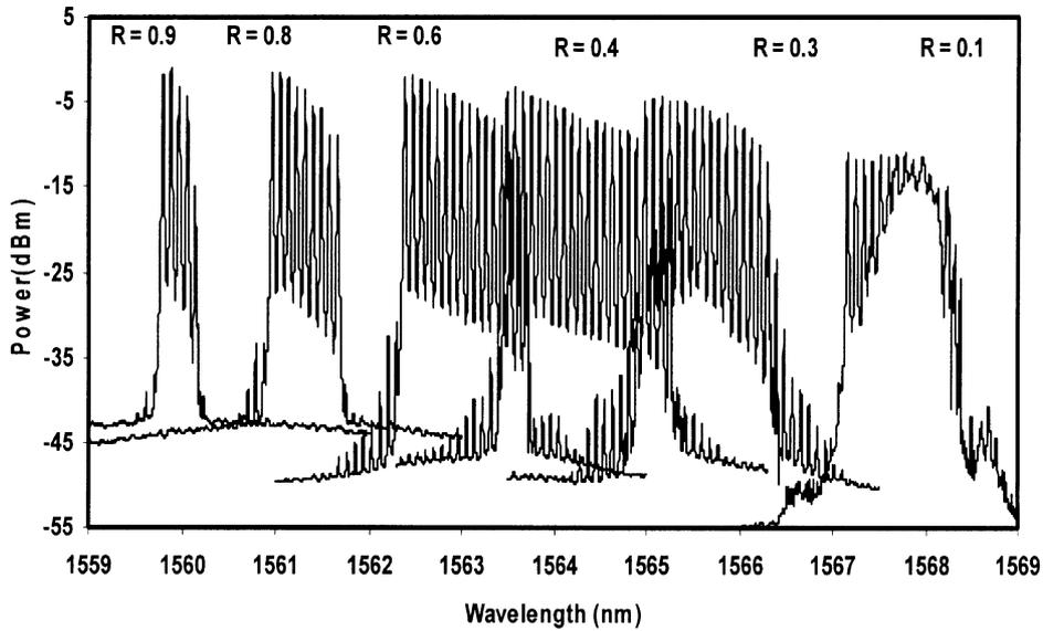
**Figure 2.** BEFL spectrum at various coupling ratios.
