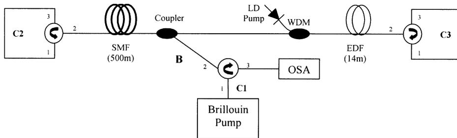
**Figure 1.** Experimental set-up of BEFL.
