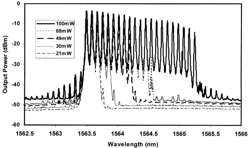
Figure 4. The BEFL spectra at various pump powers for  $R = 0.4$ .
