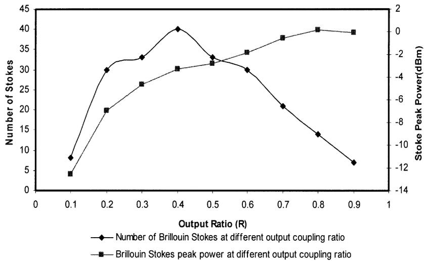
**Figure 3.** Brillouin Stokes peak power and number of Brillouin Stokes at different output ratios.
