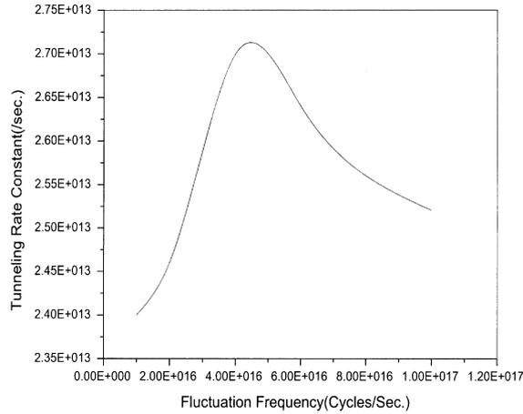
**Figure 4.** The tunneling rate constant as a function of fluctuation frequency for fixed values of barrier fluctuation strength (0.4) and coupling strength (0.01) for a classical regular subsystem.
