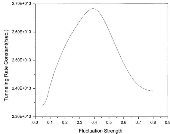
**Figure 6.** The tunneling rate constant as a function of fluctuation strength for fixed values of barrier fluctuation frequency ( $5.0E16$  cycles/s) and coupling strength (0.01) for a classical regular subsystem.
