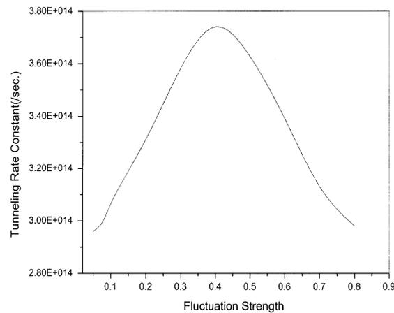
**Figure 7.** The tunneling rate constant as a function of fluctuation strength for fixed values of barrier fluctuation frequency ( $5.0E16$  cycles/s) and coupling strength (0.01) for a classical chaotic subsystem.
