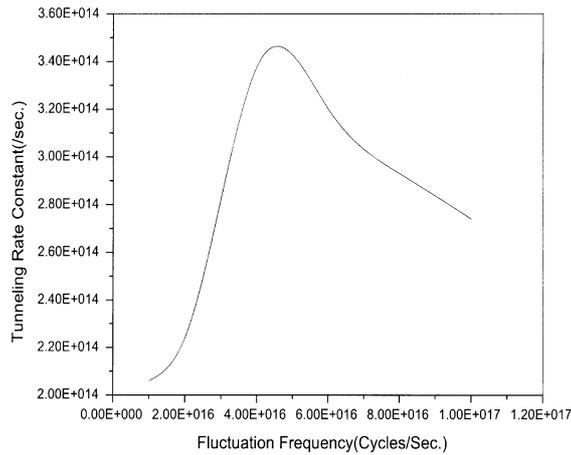
**Figure 5.** The tunneling rate constant as a function of fluctuation frequency for a fixed value of barrier fluctuation strength (0.4) and fixed coupling strength (0.01) for a classical chaotic subsystem.
