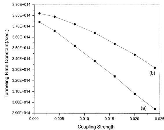
**Figure 3.** The tunneling rate constant as a function of coupling strength when the classical subsystem is chaotic (a) for fluctuating barrier (fluctuation strength = 0.4 and fluctuation frequency = 5.0E16 cycles/s) and (b) for static barrier.
