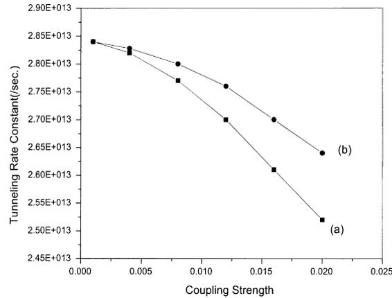
**Figure 2.** The tunneling rate constant as a function of coupling strength when the classical sub-system is regular (a) for fluctuating barrier (fluctuation strength = 0.4 and fluctuation frequency = 5.0E16 cycles/s) and (b) for static barrier.
