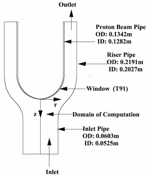
Figure 3. Schematic of the computational domain.
