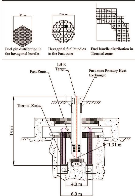
**Figure 2.** Schematic of 750 MW (thermal) one-way coupled ADS.
