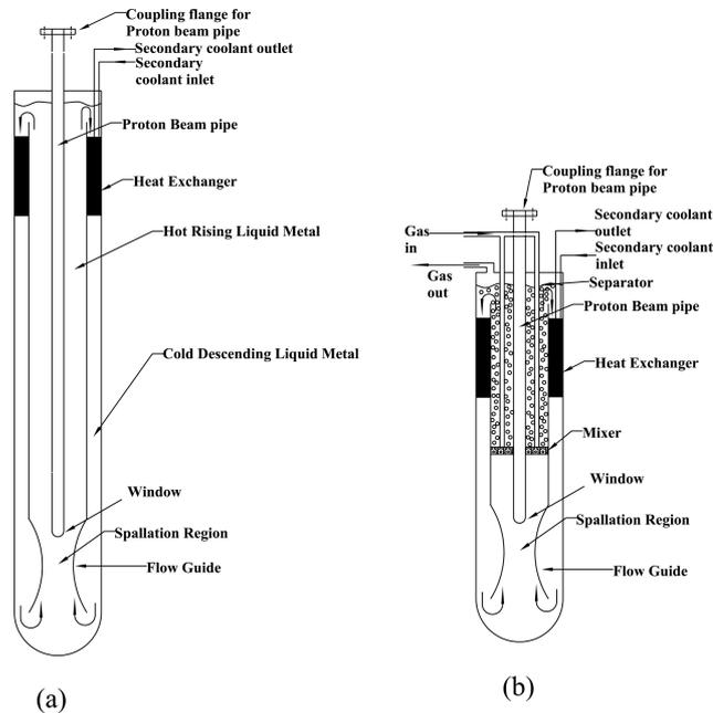
Figure 1. (a) Buoyancy- and (b) gas-driven window target module.
