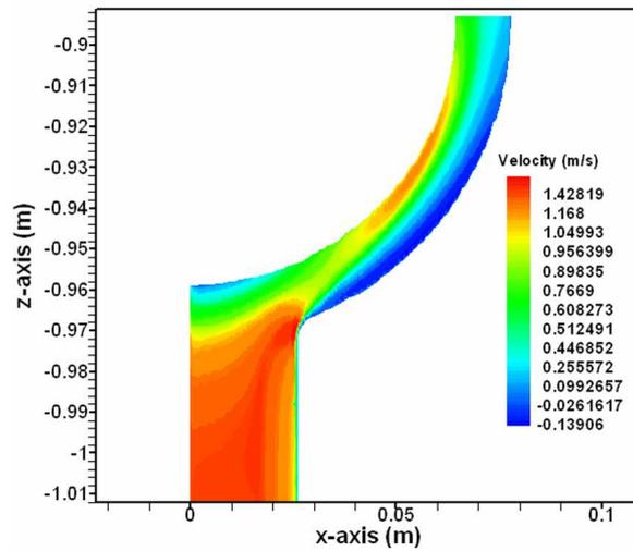
**Figure 5.** Velocity contours for 30 kg/s flow rate in geometry with smaller transitional annular radius (13.8 mm) for a proton beam of 30 MeV energy and 0.267 mA beam current.
