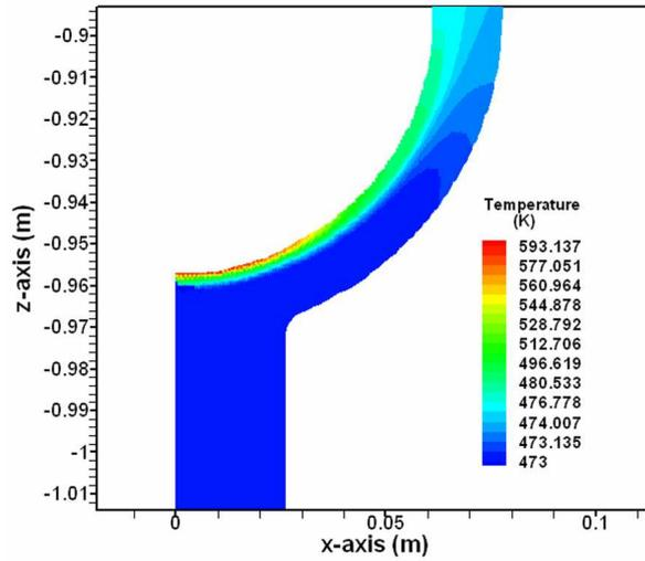
**Figure 4.** Temperature contours for 30 kg/s flow rate in geometry with smaller transitional annular radius (13.8 mm) for a proton beam of 30 MeV energy and 0.267 mA beam current.
