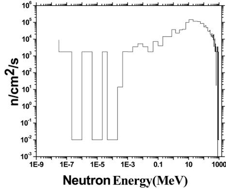
**Figure 1.** Fluence passing through the Ta-sample placed at the circular downstream face (outer side of paraffin) at  $20^\circ$  to the line joining the two paraffin dees.
