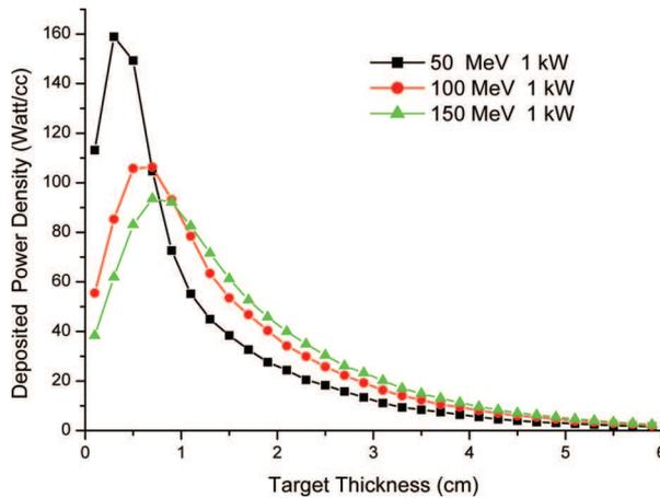
**Figure 4.** Heat deposition density as a function of target thickness for different incident electron energies (1 kW power).
