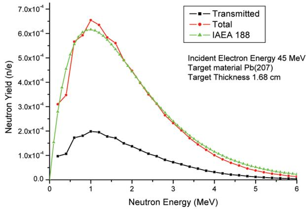
Figure 1. Comparison of neutron spectrum from lead target.
