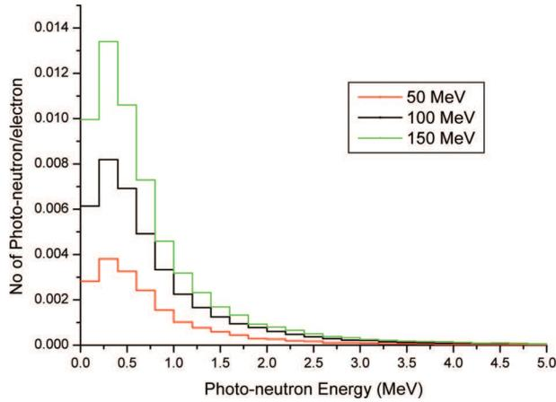
**Figure 5.** Photoneutron energy spectrum from Ta target.
