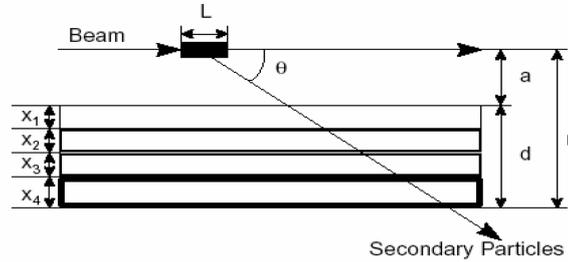
**Figure 1.** Shield geometry.
