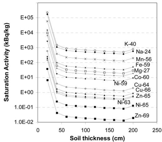
**Figure 3.** Saturation activity of different radio-nuclides formed by neutrons at different soil thicknesses due to 1 mA protons on LBE.
