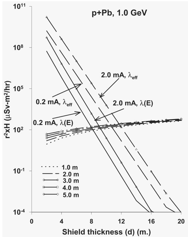
**Figure 2.** Transmitted dose through different shield thicknesses and the regulatory limits (horizontal curves), both multiplied by  $r^2$  (the square of the distance from the target).
