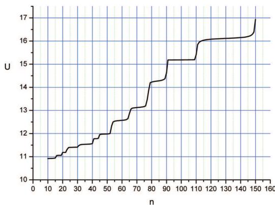
**Figure 1.** A typical non-uniform splitting of lethargy scale  $U(n)$  for the PWR pin cell,  $n$  – number of groups.
