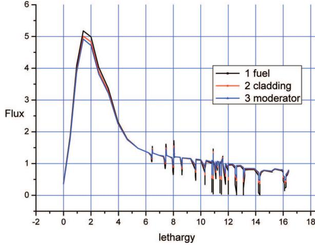
**Figure 2.** A typical flux distribution depending on lethargy (in 3 zones of PWR pin cell with MOX fuel) .
