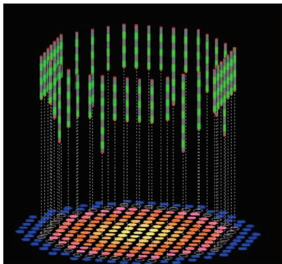
**Figure 3.** An example of power distribution and CR positions in the process of 3D burnup simulation (a model of fast lead-cooled reactor).
