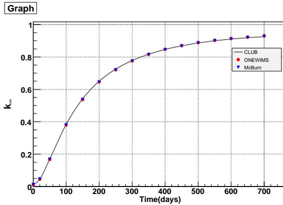
Figure 2. Comparison of McBurn and ONEWIMS (of the BURNTNAN package) with CLUB for PHWR lattice cell with 19-rod Th cluster.
