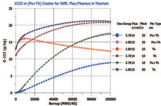
Figure 8. Variation of  $^{233}\text{U}$  with burnup in Pu+Th cluster for different flux/fluence in thorium.
