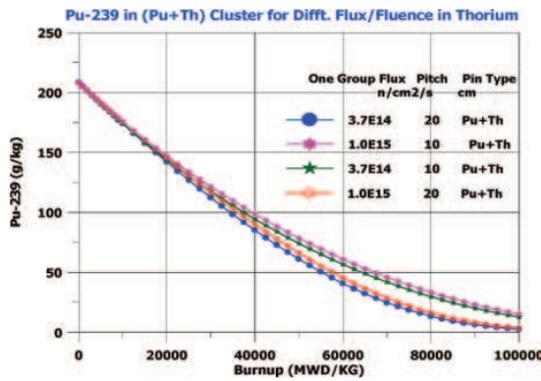
Figure 9. Variation of  $^{239}\text{Pu}$  with burnup in Pu+Th cluster for different flux/fluence in thorium.
