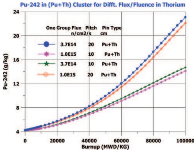
Figure 12. Variation of  $^{242}\text{Pu}$  with burnup in Pu+Th cluster for different flux/fluence in thorium.
