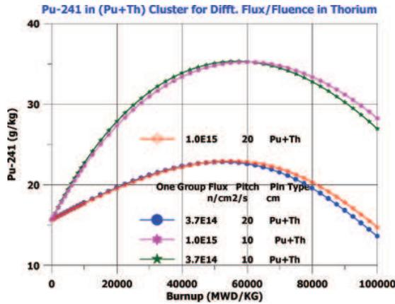
Figure 11. Variation of  $^{241}\text{Pu}$  with burnup in Pu+Th cluster for different flux/fluence in thorium.
