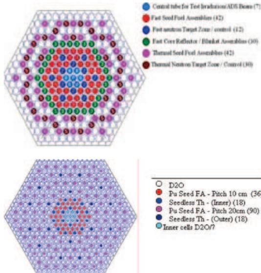
Figure 2. (a) Tentative HFTR 100 MWt core layout-1. (b) Tentative HFTR 100 MWt core layout-2.
