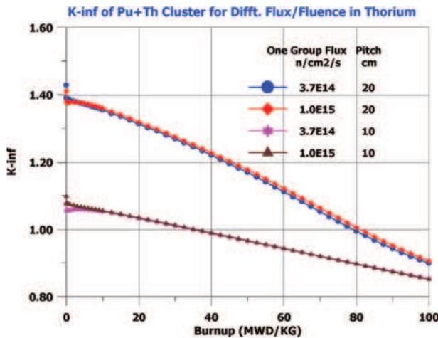
Figure 7. Variation of  $K_{\infty}$  with burnup in Pu+Th cluster for different flux/fluence in thorium.
