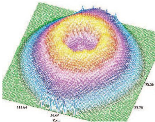
Figure 3. Thermal flux distribution at the core mid-plane.
