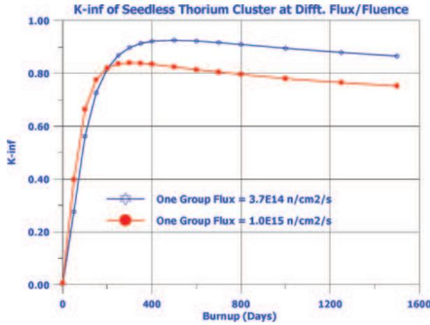
Figure 6. Variation of  $K_{\infty}$  with burnup in Th cluster at different flux/fluence.
