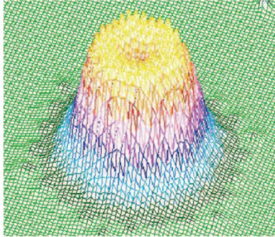
Figure 4. Fast flux distribution at the core mid-plane.
