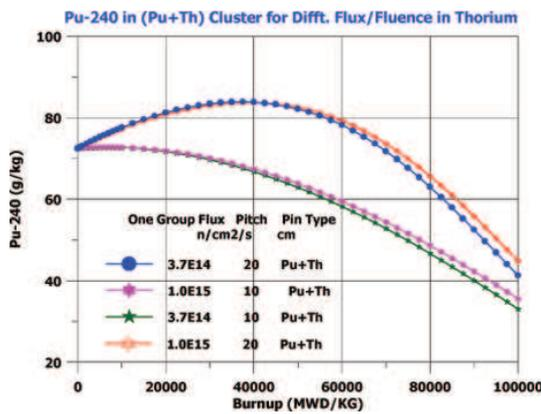
Figure 10. Variation of  $^{240}\text{Pu}$  with burnup in Pu+Th cluster for different flux/fluence in thorium.
