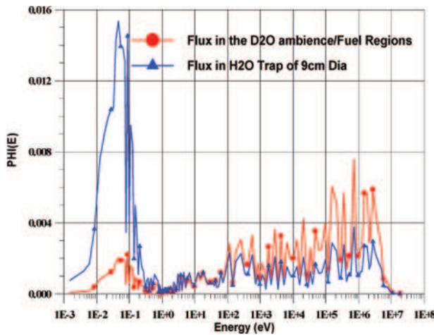
Figure 5. Enhancement of thermal flux by annular H<sub>2</sub>O in D<sub>2</sub>O.
