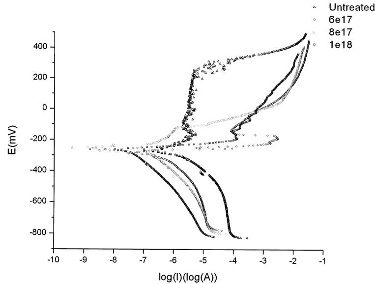
**Figure 3.** Potentiodynamic polarization curves acquired from the AISI 304 in 3 wt% NaCl solution for different doses.
