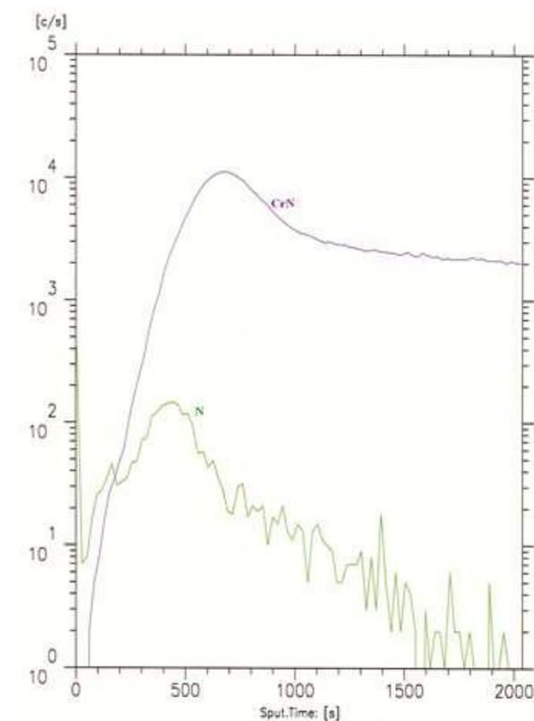
**Figure 2.** SIMS depth profile of nitrogen and CrN corresponding to the dose of  $8 \times 10^{17}$  ion/cm<sup>2</sup>.
