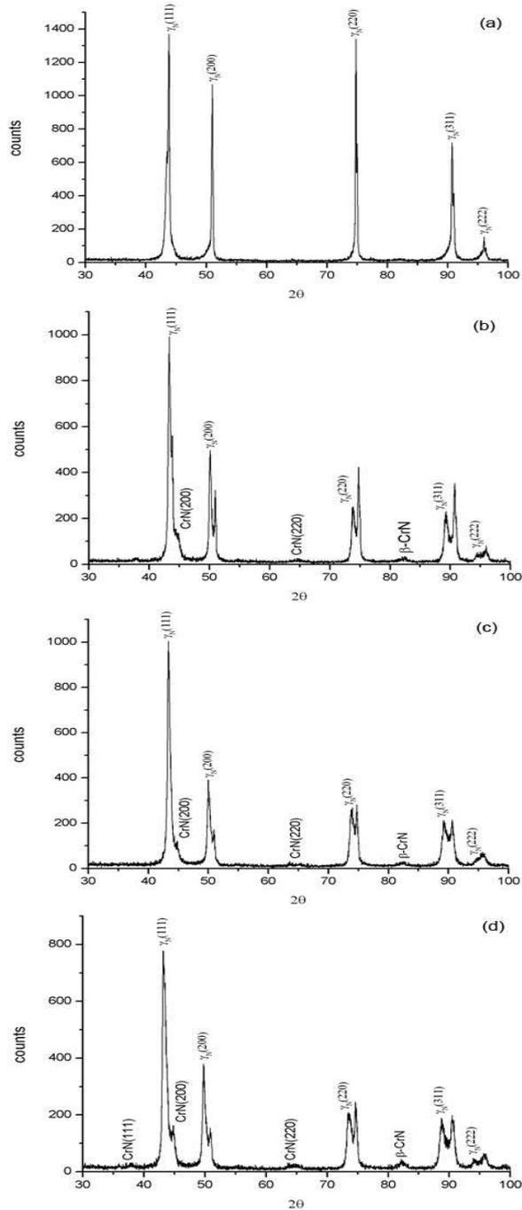
Figure 1. XRD patterns for (a) untreated sample and different doses of (b)  $6 \times 10^{17}$  ion/cm<sup>2</sup>, (c)  $8 \times 10^{17}$  ion/cm<sup>2</sup> and (d)  $1 \times 10^{18}$  ion/cm<sup>2</sup>.
