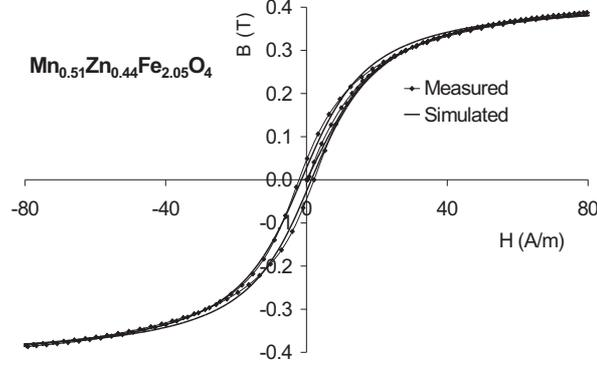
**Figure 1.** Magnetic hysteresis loop  $B(H)$  of Mn–Zn ferrite measured and calculated from the model.
