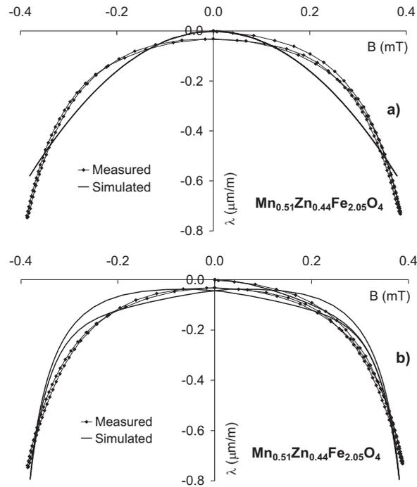
**Figure 3.** Magnetostrictive hysteresis loop  $\lambda(B)$  of Mn–Zn ferrite measured and calculated from the model. (a) Quadratic dependence, (b) J–A–S model.
