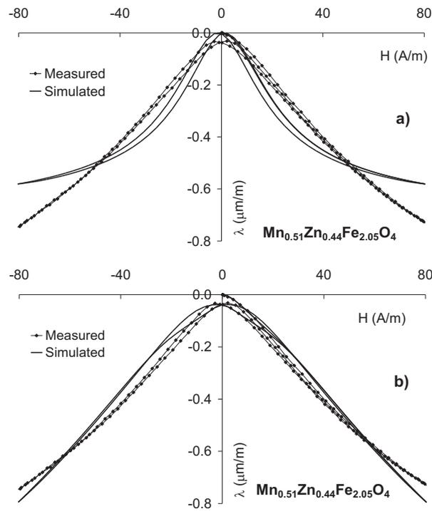
**Figure 2.** Magnetostrictive hysteresis loop  $\lambda(H)$  of Mn–Zn ferrite measured and calculated from the model. (a) Quadratic dependence, (b) J–A–S model.
