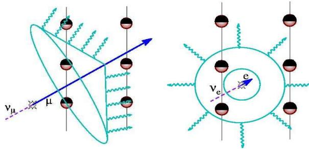
**Figure 1.** Left: Schematic of  $\nu_\mu$ -induced muon track in detector. Right: Schematic of  $\nu_e$  cascade.
