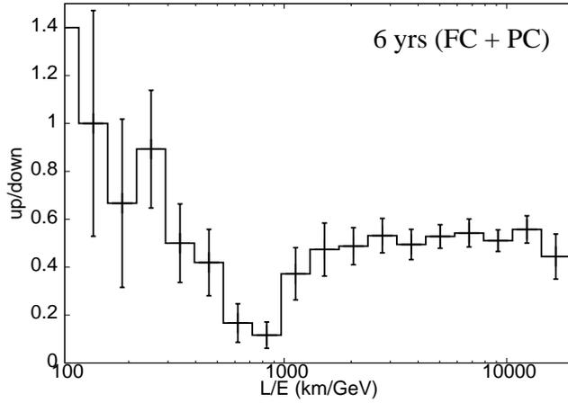
**Figure 2.** The ratio of upward-going to downward-going muon events for six years of data simulation. The input values are  $|\Delta_{31}| = 2 \times 10^{-3} \text{ eV}^2$  and  $\theta_{23} = 45^\circ$ . The position of the dip is sensitive to the magnitude of  $\Delta_{31}$  whereas the value of the ratio at the dip is sensitive to  $\sin^2 2\theta_{23}$ .
