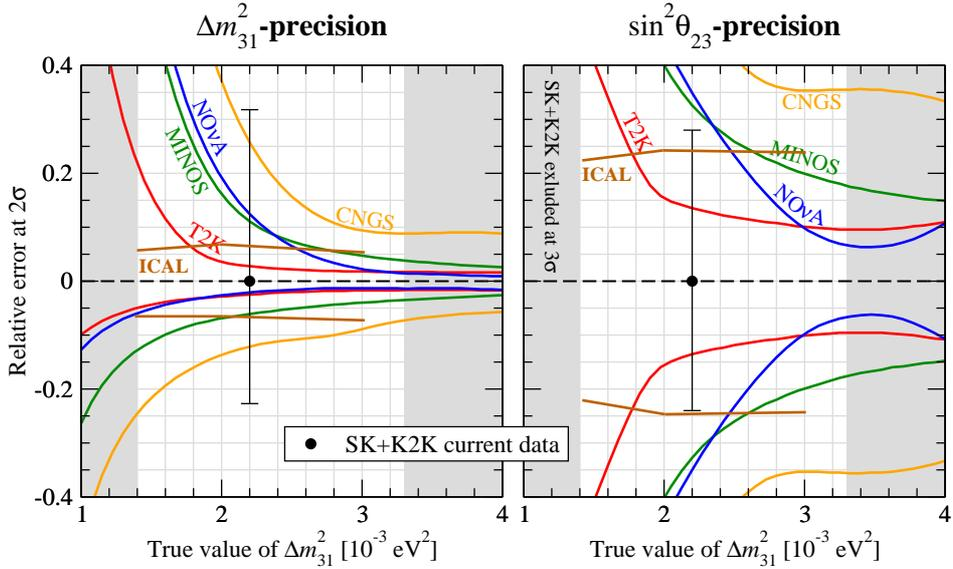
**Figure 3.** The relative error on  $|\Delta_{31}|$  and  $\sin^2 \theta_{23}$  as a function of the input value of  $|\Delta_{31}|$  at  $2\sigma$  level. The figure is adopted from P Huber *et al*, hep-ph/0412133, with the curve for ICAL overlaid.
