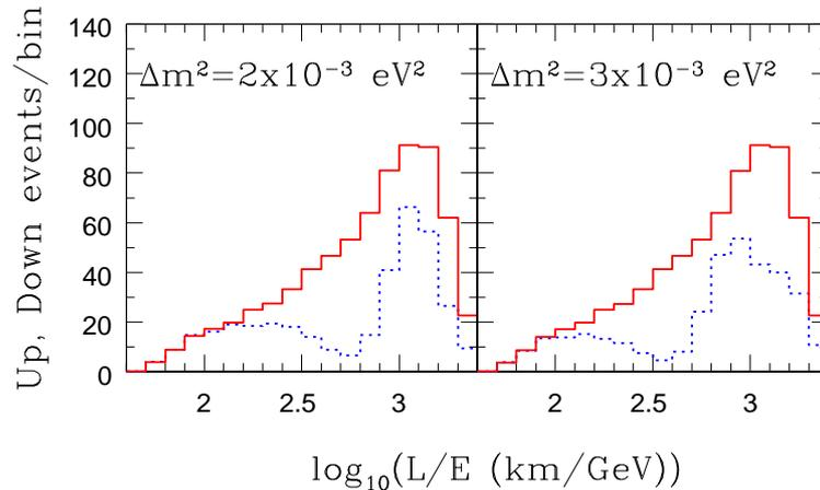
**Figure 1.** The number of upward-going (broken histogram) and downward-going (solid histogram) muons (of either sign) in  $(L/E)$  bins are presented for  $|\Delta_{31}| = 0.002 \text{ eV}^2, 0.003 \text{ eV}^2$  and  $\theta_{23} = \pi/4$  for an exposure of 250 kton-yr at ICAL.
